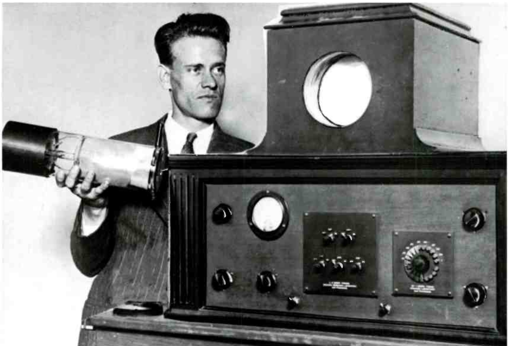
These two men perfected the all-electronic television system, which displaced the mechanical scanner. Philo T. Farnsworth ( below ), developed the "dissector tube," an electronic alternative to the mechanical disassembling and reassembling of pictures, and Vladimir K. Zworykin ( left ), developed the iconoscopic camera and the kinescopic receiving tube. These devices made it possible to transmit and receive television pictures instantaneously, through the use of electrical signals.
