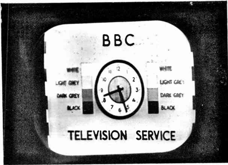
Picture too narrow. Adjust picture width control until the clock is circular. Slight adjustment of the line linearity control is also necessary as there is evidence of slight cramping on the left
