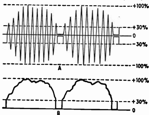
Fig. 27—The form of the signal as it leaves the I.F. amplifier is shown at A; at B is the same signal after passing through the demodulator stage
