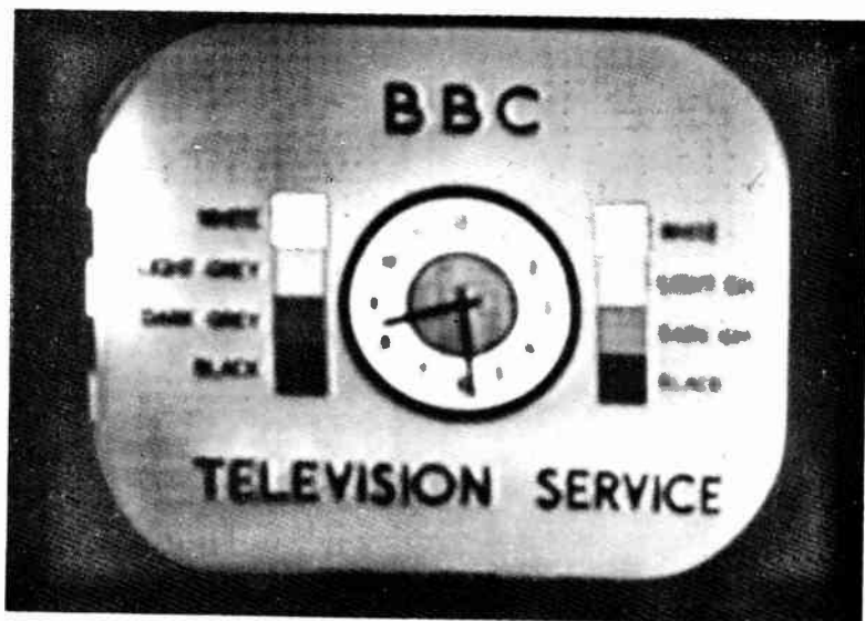
Picture out of focus and too contrasty. Adjust focus control, reduce contrast control and increase brightness control settings
