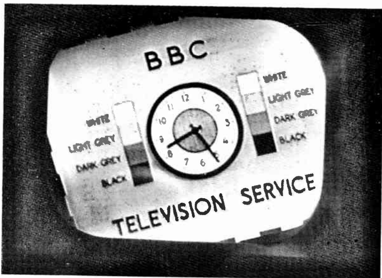
Picture not horizontal. Adjust mechanical control inside the receiver which rotates the scanning coil unit
