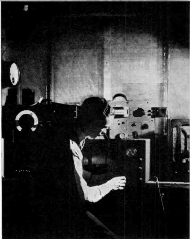
Engineers check up the tonal qualities of a radio receiver and make sound visual on this oscilloscope for close study
