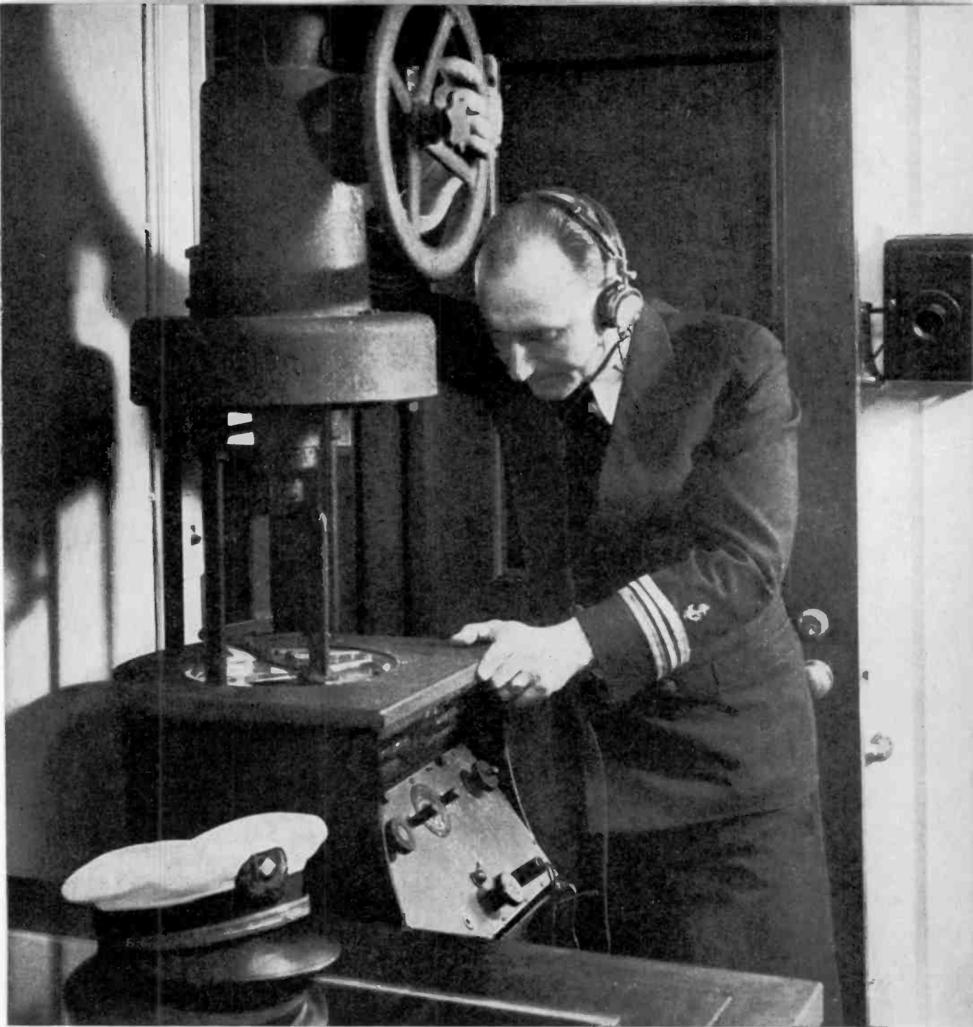
The ship's officer takes a bearing on the radio direction finder
