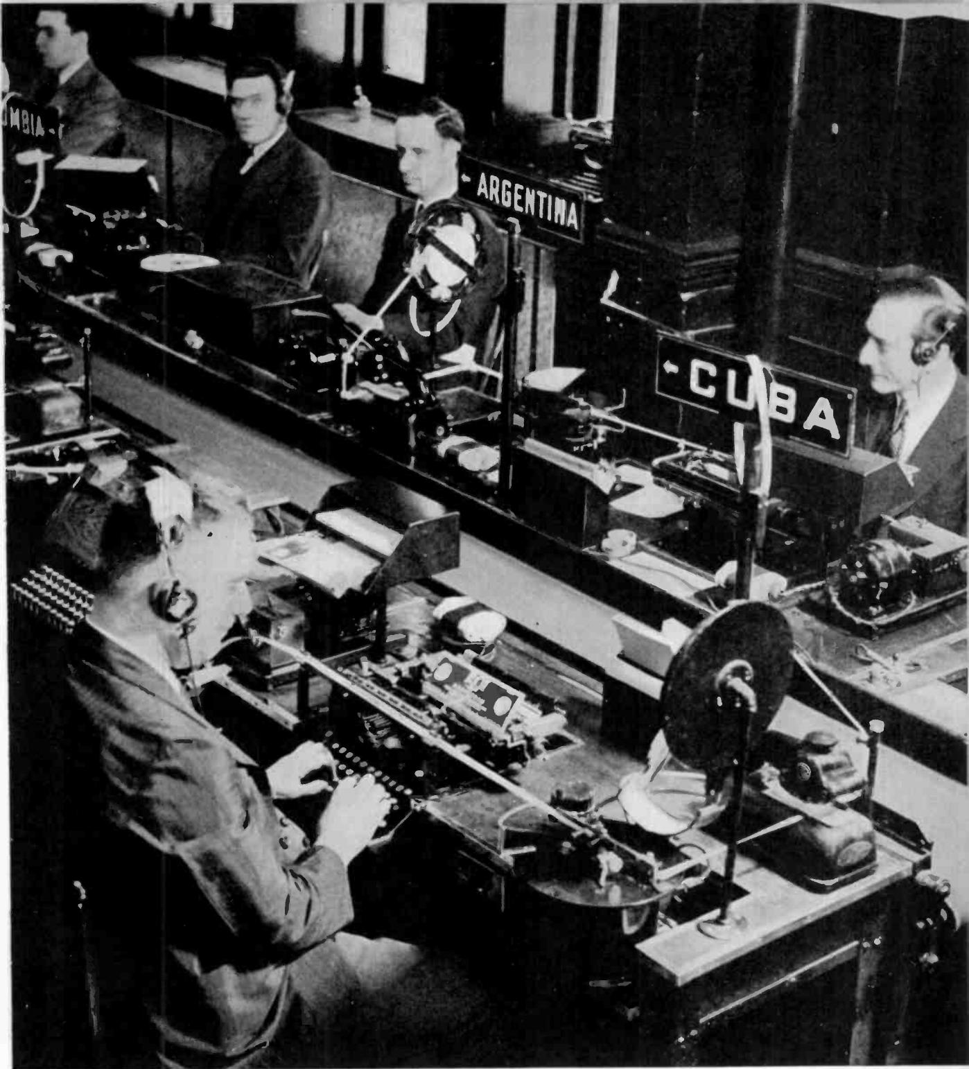
The operator in the foreground is transcribing the wavy line on a receiving tape into the words of a message
