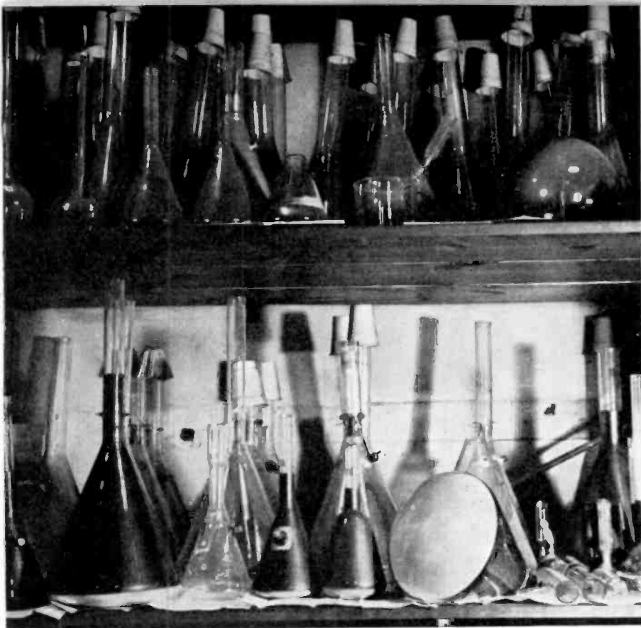
Experimental cathode ray tubes waiting to receive their electron guns. The tube at lower right shows the fluorescent material on the flat end
