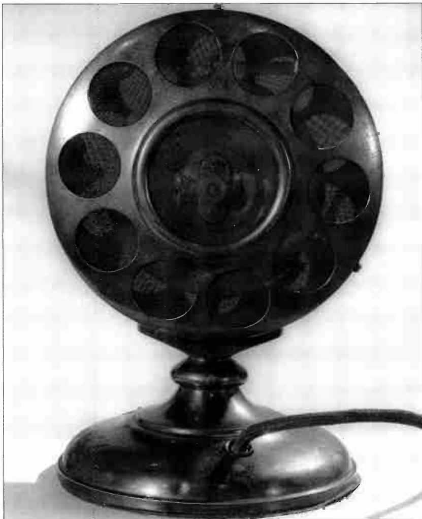
The two-button carbon microphone was used in most radio stations in the 1920s. Sometimes Les Spencer had to hit it on the back to keep it working.
