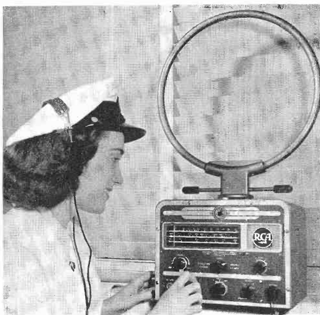
Radio direction finders first came into general use during World War I and, since that time, have been developed for service on small craft as well as on ocean liners and airplanes.
