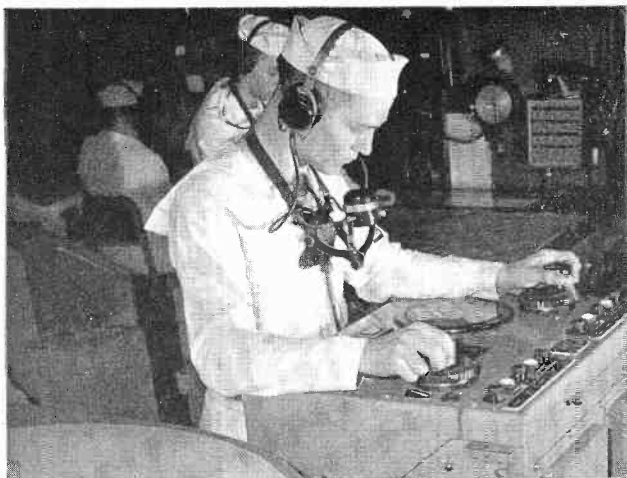
Radar: Ra-radio; d-detection or direction-finding; a-and; r-ranging, added a new dimension to direction finding and navigation at sea and in the air during World War II. (U. S. Navy Photo.)
