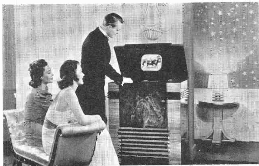
The popular television set, first introduced by RCA for public use at the New York World's Fair in 1939, featured a picture reflected from the top of the kinescope to a mirror on the underside of the cabinet's uplifted lid.
