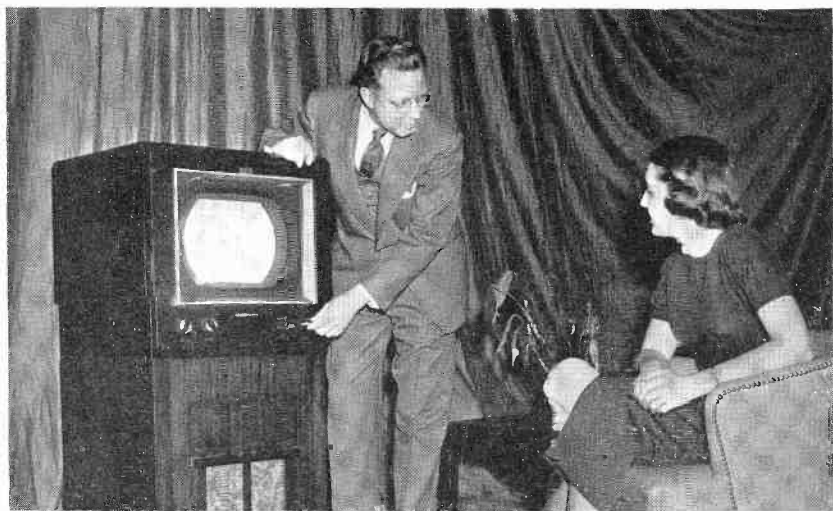
All-electronic color television receiver, demonstrated by RCA for the first time publicly in March 1950, introduced a new direct-view color picture tube.
