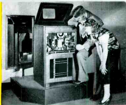
RCA television receiver with front panel removed to show the interior.
