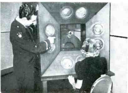
Outmoded mechanical scanning camera. Subject sat before photoelectric cells.
