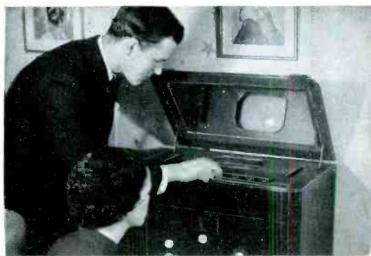
Close-up of receiver; Kinescope image is reflected onto mirror under lid.
