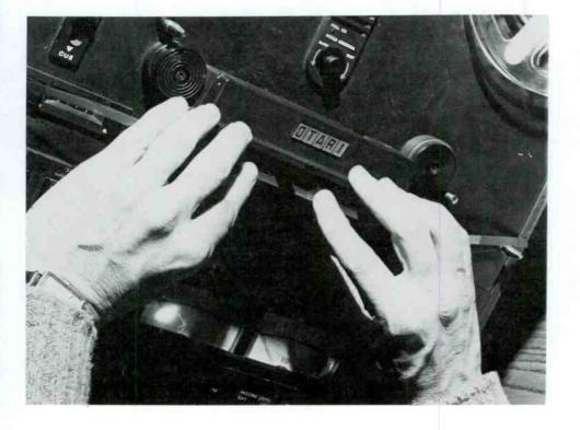
FIGURE 9.26E Place a 3/4-inch-long piece of splicing tape against the nonrecording surface of the magnetic tape.
