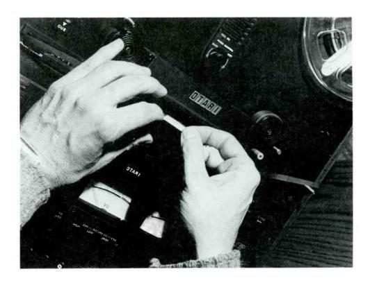
FIGURE 9.26F Remove the air bubbles trapped between the splicing and magnetic tapes by gently rubbing the surface. Tape must adhere completely to ensure permanent grip.
