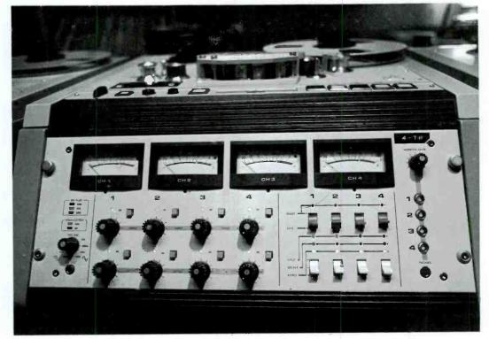
FIGURE 9.11 Four-track reel-toreels are the most common multitrack recorders at radio stations. Courtesy WMJX-FM.
