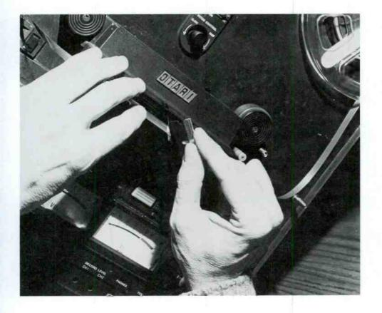
FIGURE 9.26C Make a diagonal cut with a single-edge razor. Use a sharp razor to avoid uneven cut.
