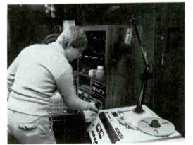
FIGURE 9.24 Production director setting levels for dubbing purposes. The foam windscreen on the microphone helps prevent distortion.
