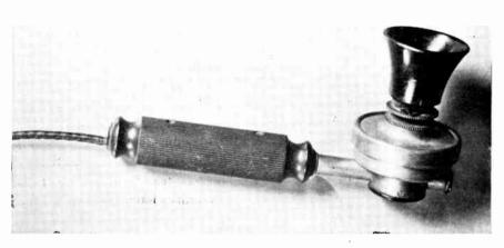
FIGURE 18. One of the first devices used to get a realistic "filtered" telephone effect. The actor spoke into the hand-held phone instead of speaking into a filtered cast mike. (Courtesy of National Broadcasting Company.)
