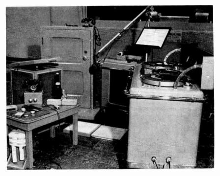
FIGURE 23. Sound setup for one soundman showing placement of cardioid mike. (Courtesy of Don Lee Broadcasting System.)
