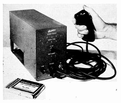
FIGURE 21. Aeronic's Sono-shot, an instrument that simulates live gunshots by electronically firing shotgun primers. (Courtesy of Aeronics, Inc., of New York.)
