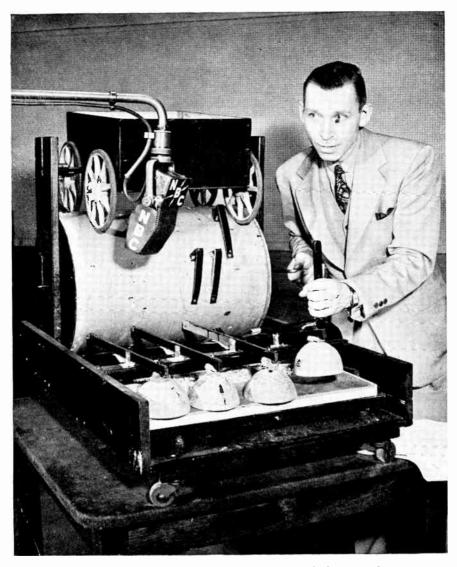
FIGURE 9. Soundman Tommy Evans operating NBC's horse and wagon apparatus. The eccentric offsets on the revolving drum activate the hooves in proper rhythm. Surfaces under the hooves are interchangeable to simulate different terrain. (Courtesy of National Broadcasting Company.)
