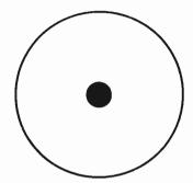
The small circle indicates the nondirectional mike. The large circle indicates the pickup pattern. Any sound given on the periphery of the large circle will have the same volume and frequency response, no matter from what direction it comes. In other words, the pickup is not limited to any specific direction; the beam is 360 degrees; there is no dead side. If used for sound, a nondirectional mike should be mounted so that the axis of the beam is parallel to the floor.
