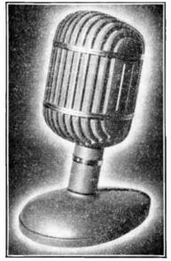
Fig. 24. Western Electric 639B cardioid microphone, on desk-type base. Combines a dynamic moving-coil pressure element with an improved ribbon-type velocity element.
