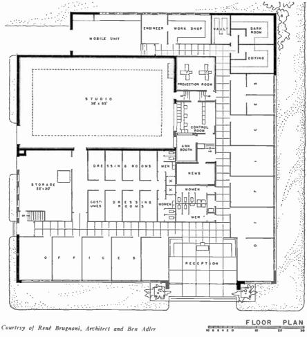
FIG. 11. Floor plan for TV station, intermediate size.
