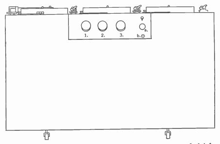
FIG. 19. *Above*, view of sound truck from top. Volume controls 1-4 for pick-up arms I-IV. A, B, C, turntables. a, dynamic noise suppressor. b, phone jack for head set monitoring. *Below*, view of sound truck from front. Volume controls 1-3, panel sloping.
