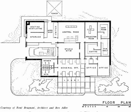
FIG. 10. Floor plan of a small TV station.
