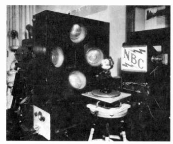
During the early experiments with electronic television, RCA laboratories used, as a moving object to televise, a 12-inch paper maché model of a popular cartoon character, Felix the Cat, posed on a revolving turntable under hot lights. The image at left shows how Felix looked on television in 1929 when picture definition was still only 60 lines per frame.
