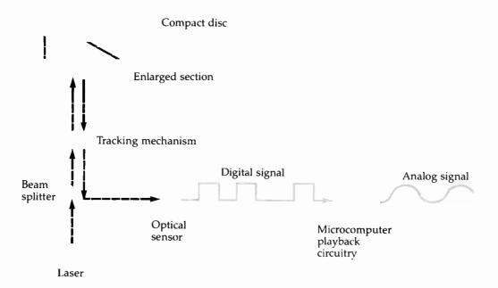
Sound has been recorded on the revolving disc in the form of microscopic pits representing a digitally encoded version of the original signal. A laser beam, guided by a supersensitive tracking mechanism, strikes the pits; they reflect the beam back as a modulated digital signal to an optical sensor. The sensor feeds its digital output to a microcomputer that has a transducer for converting the digital information into analog form for delivery to the audio reproducing system.
