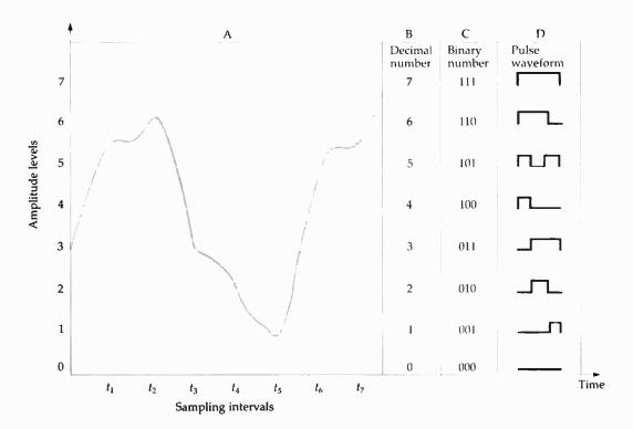
each point. Note that the digital wave, depicted in column D, can have only two conditions, either "on" or "off," with the *time* as an additional variable. Continuous "on" for the entire time period allotted to one item represents the binary value 111; continuous "off" for the entire period represents 000. To represent the binary number 101, the wave shows "on," "off," and another "on" within a single time segment.
