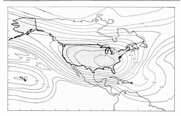
A satellite's usable coverage area, known as its footprint, is depicted on a map in terms of various levels of signal strength. The inner contour defines the satellite's boresight, its area of maximum signal strength, where the smallest receiving antennas can be used. The outermost contour defines its beam-edge power, the region beyond which satisfactory reception cannot be expected even with large receiving antennas. The numbers associated with contour lines are signal-strength measurements.
