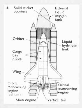
A critical moment in the life of every satellite occurs when it first leaves the Earth. Dwarfed by the enormous launch rocket(s) needed to overcome gravity and atmospheric resistance and to attain escape velocity, the fragile satellite starts its journey as a mere passenger. Only after it reaches an elevation of about 200 miles does a satellite ignite its own rocket motor to loft itself into geosynchronous orbit.
