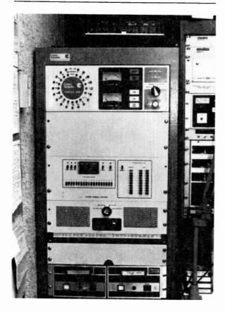
Automated tape cartridge (CART) machines help keep radio stations operating with limited staff. A combination of timing devices and carts pre-recorded with announcements, commercials, and music can provide entire dayparts. This machine, a central part of a Kansas network, can receive newscasts from other network stations for playback at late times.
