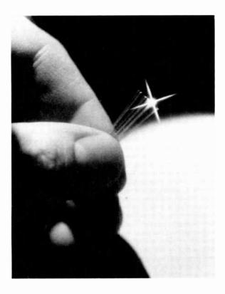
An AT&T fiber-optic cable made up of five pairs of bairthin glass strands teach pair can carry about 50,000 telephone calls) transmitted on beams of laser light. Capacity is limited not by the small size of the fibers but by the speed of the lasers that generate the information-bearing light beams and the light detectors at the receiving end. Currently, these components can send and receive 3.4 billion bits of information per second.
