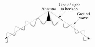
Direct waves travel straight out, like light, from small radiating elements atop an antenna support. Television antennas radiate their waves downward toward the reception area, blocking off radiation that would otherwise travel upward and outward into space. The distance to the apparent borizon limits the coverage area of direct-wave transmissions. One speaks of the "apparent" borizon because its distance varies in accordance with the beights of the sending and receiving antennas.
