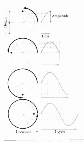
Tracing the rise and fall of a spot on the rim of a revolving wheel illustrates the concepts of cycle, phase, amplitude, and velocity. The spot starts at the level of the axle and moves first up, then down, then up again. The changing distances of the spot above and below the axle level represent changes in amplitude.
