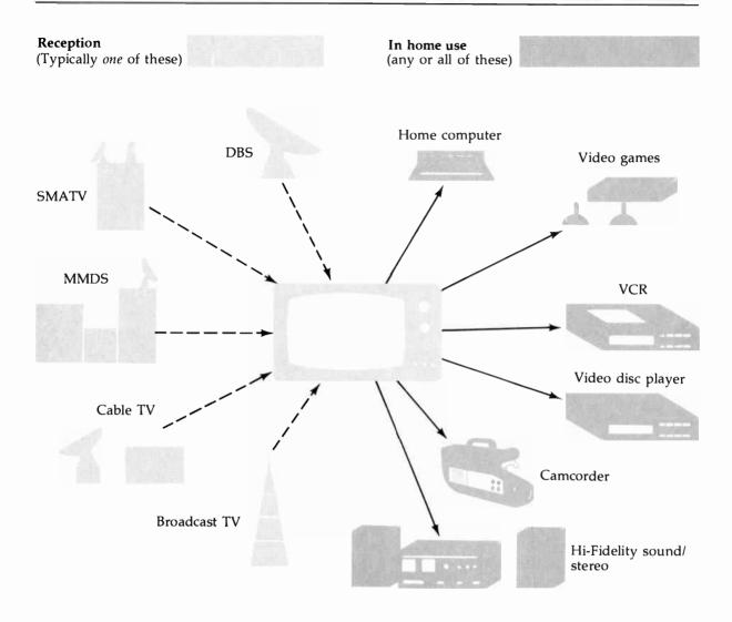
By the late 1980s, the home television receiver became the reception center for an increasing variety of video distribution channels (left side of diagram—typically only one reception unit being used per household); and in-home inputs (right side of diagram—several, if not all, devices are often connected with the one reception set).
