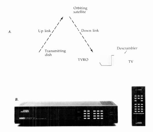
(A) Satellite delivery of programs directly to viewers' bomes depends on a reliable means of scrambling the video and sound signals, to be descrambled by devices supplied only to bomes that pay monthly subscription charges for the service. (B) The descrambling device, in this case a VideoCipher II along with its band-held remote control unit, the industry standard in the late 1980s, is installed between the viewer's TVRO and the television receiver.
