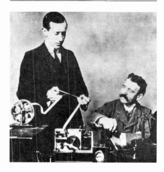
In a 1902 photo, the inventor examines the paper tape bearing a radiographic message in Morse code. Though radio equipment still remained very crude, well-developed wire telegraphy equipment could be readily adapted to record wireless messages. Seated is George Kemp, Marconi's most trusted engineering assistant.
