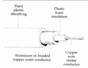
Coaxial cable gets its name from the fact that it has two conductors with a common axis: a solid central conductor surrounded by a tubelike hollow conductor. The radio energy travels within the protected environment of the space between the two conductors. Cable television relies on this type of conductor, as do many terrestrial relay links that convey television signals, telephone calls, data, and other types of information.
