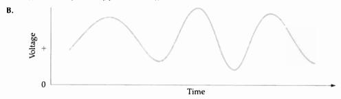
The transmitter imposes this positive voltage pattern on the carrier wave, modulating it, or causing formation of an envelope that outlines the shape of the original audio waveform. The lower half of the modulated carrier mirrors the upper half, the two balves constituting sidebands that extend above and below the carrier frequency. Note that in order to form an envelope, the carrier frequency must be higher than the baseband frequency.
