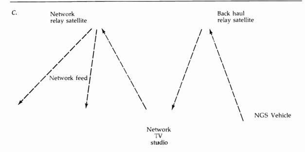
C. Using satellite relays to send program material from a new site back to the studio is called backhauling. When a broadcast network broadcasts a live on-the-spot event, it backbauls the coverage from an NGS vehicle to the studio, using leased short-term satellite capacity. From the studio, the program goes to the network's satellite uplink facility, and then to the permanently leased or owned satellite transponder that relays the program to the network's affiliates throughout the country.
