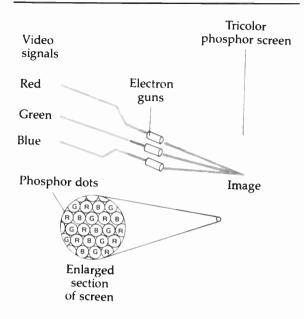
Some receiver tubes use three electronic guns and tricolor phosphor dots. Varying amplitudes in the modulated currents fed to each of the electron guns cause the dots to glow with varying intensities; though only the red, green, and blue primary colors appear on the kinescope face, the eye blends them together to make all the various bues.
