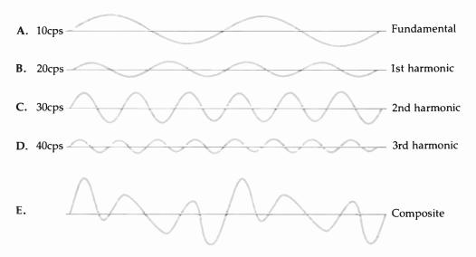
A method called Fourier analysis can be used to break down a complex wave into its component frequencies. For example, a Fourier analysis of the complex wave E yields the simple waves A through D. Wave A represents the fundamental frequency of the complex wave, vibrating at 10 cycles per second (11z). Waves B, C, and D represent harmonics of that fundamental, waves with frequencies of 20, 30, and 40 Hz, respectively. Waves A through D combined produce the composite wave E.
