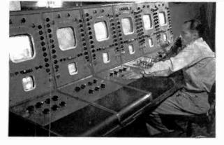
21. "Shading Desk" at WRGB. Three screens show what each studio camera is seeing, the next two what the movie and slide projection cameras are seeing, and the last the picture actually being broadcast. (Photo by courtesy of General Electric Company.)
