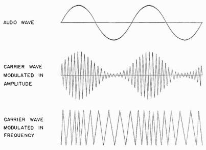
Figure 4. AM and FM Modulated Waves.
