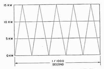
Figure 2. Line Representation of 5 KC, 10 KW Wave.
