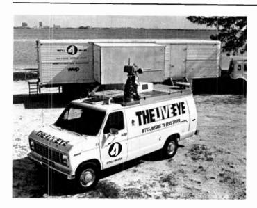
A. The unwieldy remote vehicle in the background contrasts with the compact, lightweight ENG (electronic news-gathering) van in the foreground. The machine-gun-like object on top of the van is an antenna for relaying pictures to the studio by means of microwaves.
