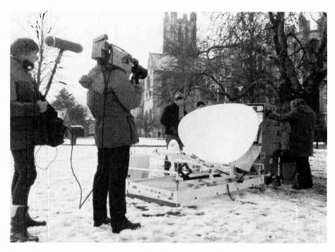
Figure 83 Portable ground-stations are used to beam news reports into space, where they are bounced off satellites and relayed to transmitters the other side of the world (courtesy ITN)
