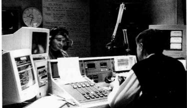
Standard equipment will include a control desk; two or more compact disc players (or record decks); cassette and DAT machines; large monitor loudspeakers; telephone and mini-switchboard system; talkback (a form of intercom); presenter and guest mikes; studio clock with on-air lights and some device for playing audio clips and jingles.
