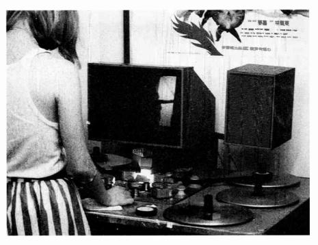
Figure 92 The Steenbeck flatbed editing machine permits the editor to review the film on screen while listening to the soundtrack (Andrew Boyd)
