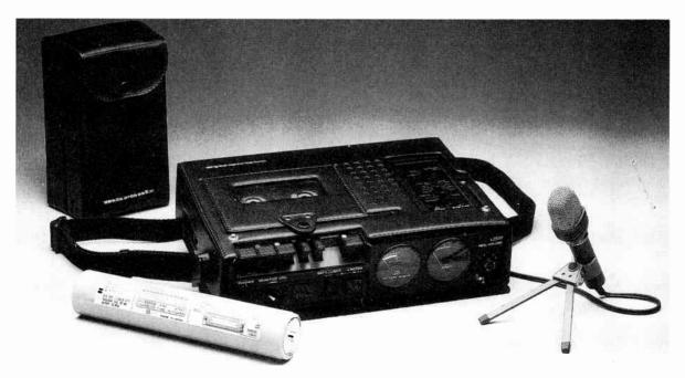
It has a *tape selector* to set the correct bias and equalisation for the cassette tape. *Normal* is used for ferric oxide tapes, *Cro2* for aluminium dioxide and similar, and *metal* for metal tapes.
