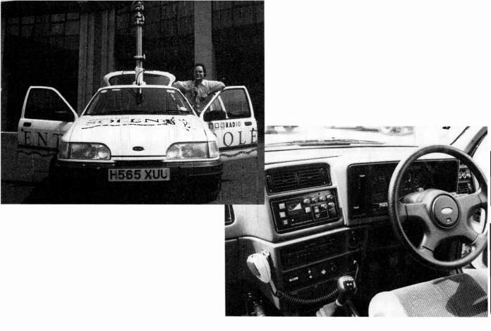
**Figure 44** (*Left*) The radio car with its tall pump-up aerial acts like a mobile studio for sending on-the-spot reports back to the station. (*Right*) The idea is to keep the operation as simple as possible so that even the most non-technical of reporters can cover a breaking story without having to bring an engineer along to press the buttons (Andrew Boyd)
