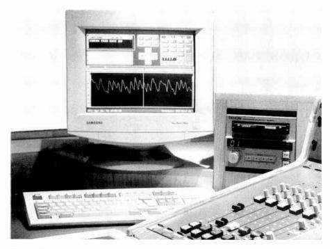
Figure 63 Sound is displayed as a waveform. The 'tape' is shuttled back and forth by clicking on a button on the screen. Cutting and pasting is carried out electronically without a razor blade or splicing tape in sight (Andrew Boyd)
