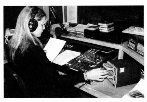
Figure 64 Self-operated news. A trainee journalist reads the bulletin and plays in all the interview clips on cartridge. This studio at the Surrey Institute is equipped with both analogue and digital cart machines. The script is held up so the paper will not rustle while the rest of the pages are kept in a blank area in the centre of the mixing desk (Andrew Boyd)
