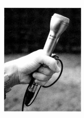
Figure 55 Mike handling. Take up the slack on the cable, being careful not to pull at either of the connections, and grip the mike lightly (Andrew Boyd)
