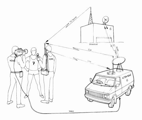
Figure 82 Live broadcasting in action. The camera sends its signal by cable to the outside broadcast (OB) van. The reporter's sound signals are sent via a transmitter carried by the reporter and aerial strapped to his shoulder. Sound and vision signals are then beamed by microwave dish to a receiver at the TV station. The reporter can hear his report going out and receive his cues from the control room via another antenna on his shoulder (courtesy Sony Broadcast Ltd)
