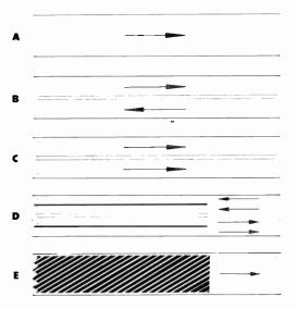
Full track. Mono recording is made across the whole width of the tape. Tape cannot be turned over
