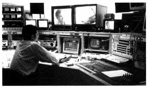
Figure 74 Inside the production suite at ITN. Computer-controlled editing lays down pictures, soundtrack and graphics directly on to the Betacam cassette (Andrew Boyd)
