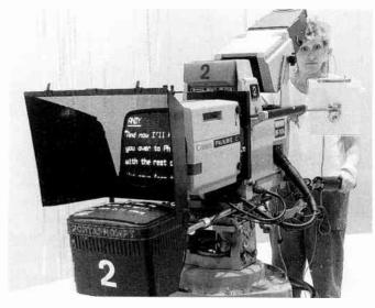
Figure 101 The camera operator takes her cue from the camera script (crib cards). The automatic prompter reflects the presenter's script on to a sheet of glass in front of the camera lens (courtesy EDS Portaprompt)
