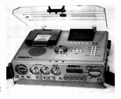
Figure 54 Recording goes solid-state. The Nagra ARES-C uses credit card sized PCMCIA cards to store up to 40 minutes of sound. Recordings can be edited on the machine and downloaded directly on to a computer (courtesy Kudelski)
