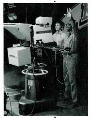
Figure 7.4. A studio camera focused on a single performer.
