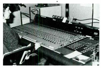
AMPLIFICATION: The electrical signal strength of most components in the radio control room is very weak, and the console must amplify these signals to a level high enough to feed the transmitter or a tape recorder.
