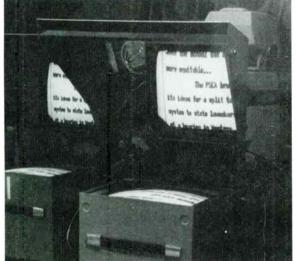
Figure 4.10. A prompting device allows you to read from the script while maintaining eye contact with the camera.
