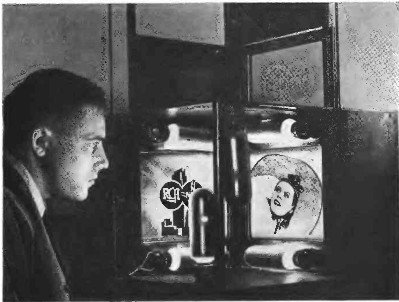
THE OPTICAL DISSOLVE TITLE MACHINE USED AT NBC
