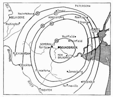
FIG. 8.—The significance of good location is shown by the lines of equal field strength measured from WJZ at Bound Brook. The figures are milli-volts per meter. (*Courtesy of the Institute of Radio Engineers.*)
