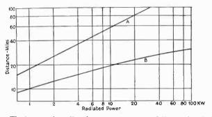
FIG. 13.—The increase in radiated power necessary to deliver a signal of 10,000 microvolts per meter over the distances indicated. Curve A assumes no absorption; Curve B gives the corresponding relations observed for suburban and country terrain. Prepared by D. R. Dept., A. T. T. Co. (Courtesy of American Institute of Electrical Engineers.)
