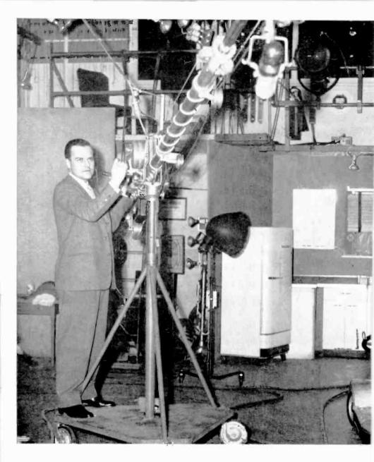
Here is the often mentioned "boom." Next to the camera, it is the most important device on the set. It is a long derrick arm on the end of which is hung the microphone that picks up voices and sounds and sends them hurtling simultaneously with the TV signal into millions of homes.
