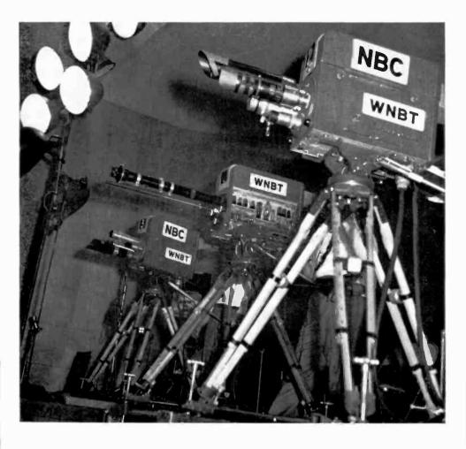
Battery of cameras in action during a TV show. These are supplemented by the more mobile dolly camera. Note telephoto lens on center camera. It is essentially a telescope that brings a distant image close to the viewer.
