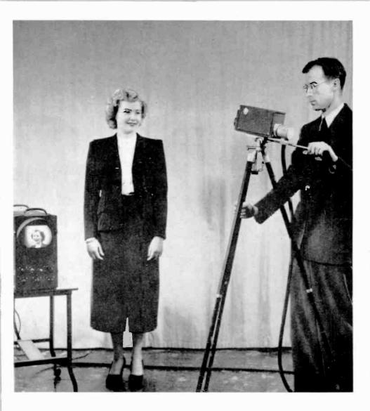
The Vidicon in use. Ensconced in a small camera, it produces the clear well-defined image seen in the portable monitor on the nearby table.
