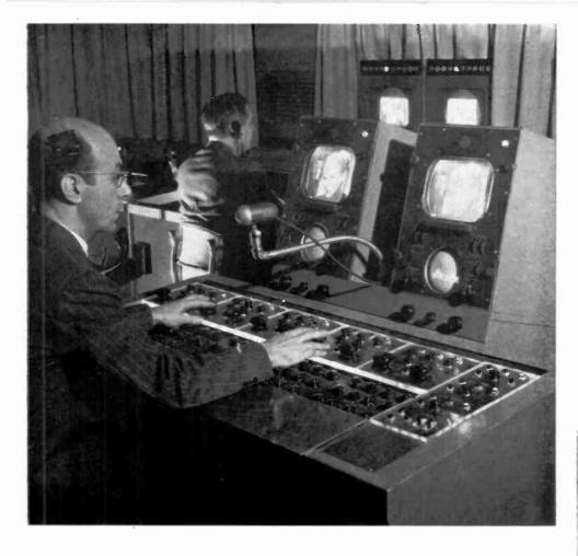
The quality of the picture as it appears on our home TV set depends largely on the skill and the knowledge of the video engineer. He is quick to correct, by means of the knobs and buttons on his desk, the slightest deviation from a clear and steady image.
