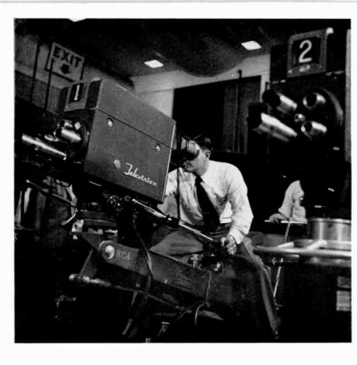
Here is the dolly camera, a kind of roaming reporter in the studio. Its huge bulk is pushed around by a "dolly man" at command of the cameraman, with whom he is connected by a complete telephone system.
