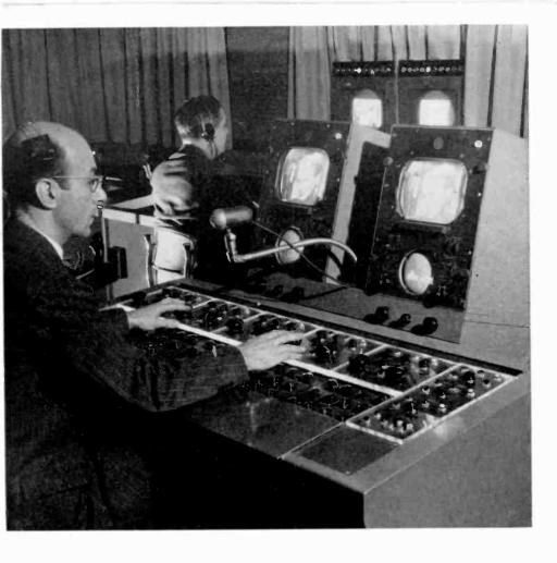
The quality of the picture as it appears on our home TV set depends largely on the skill and the knowledge of the video engineer. He is quick to correct, by means of the knobs and buttons on his desk, the slightest deviation from a clear and steady image.
