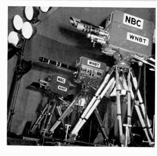
Battery of cameras in action during a TV show. These are supplemented by the more mobile dolly camera. Note telephoto lens on center camera. It is essentially a telescope that brings a distant image close to the viewer.
