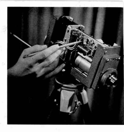
One of the miracles of television is the little Vidicon camera. Into its small bulk is compressed all the essential parts and functions of the vastly larger and more cumbersome TV camera. Because of its handy size it may be used in industry at a hundred observation posts that, through risk or expense or inaccessibility, had always gone unobserved.
