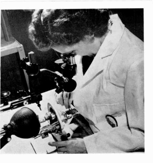
The human eye, no matter how good, is not sharp enough to fit certain parts that go into the assembly of, say an image orthicon. Here the microscope is a must.
