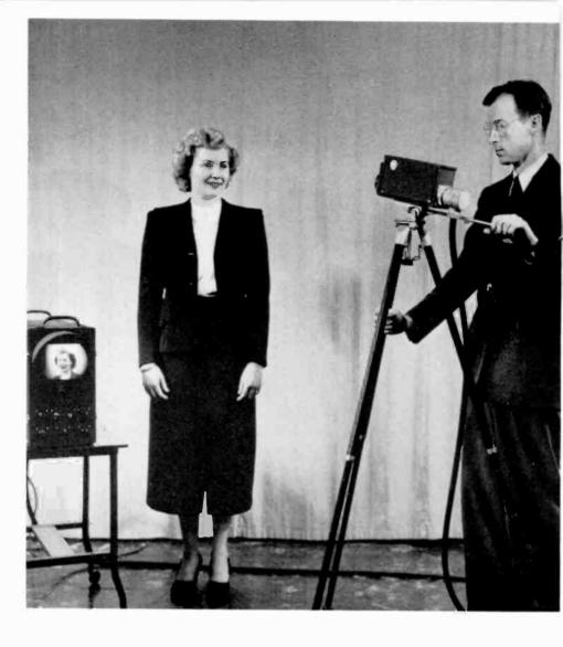
The Vidicon in use. Ensconced in a small camera, it produces the clear well-defined image seen in the portable monitor on the nearby table.
