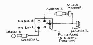
11.23 The setup of video feedback is relatively simple. Camera 1 photographs object X and feeds it into the switcher on mix bus A. This picture is fed into the studio monitor. Camera 2 photographs the studio monitor, which now displays an image of object X. Camera 2 is fed into mix bus B. Cameras 1 and 2 are now superimposed and fed as a super into the line monitor, which now shows the multiple images of object X as multiplied by the closed feedback loop between cameras 1 and 2.
