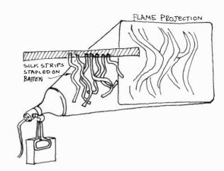
11-36 Fire: To project flickering fire onto the set, move a batten with silk strips stapled on it in front of a strong spotlight.
