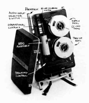
16.5 Portable Videotape Recorder: This Ampex 2-inch portable tape recorder can be carried as a backpack by the camera operator. Usually, however, the VTR is carried and operated by a second production person.
