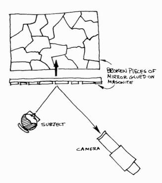
11.30 A multi-image, rosetta-like effect is achieved by mirrors reflecting each other's images, like barbershop mirrors that hang on opposite walls. Toy kaleidoscopes are based on this principle. You can duplicate the kaleidoscope effect by taping two small mirrors or ferrotype plates along one edge, so that the reflecting surfaces face each other. When the camera looks at the object that is placed in the resulting v, you will get a rosetta-like pattern of the object.
