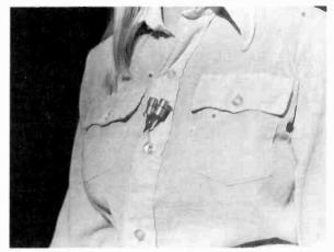
7.14 Dual-Redundancy System: A special clip permits the use of two lavalieres for dual-redundancy pickup. In case one microphone goes out, the audio engineer simply switches over to the other without losing audio. Two single clips will work in an emergency.
