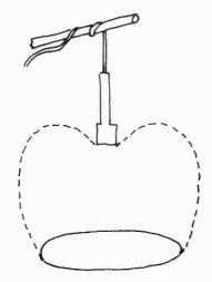
7.24 Hanging Microphone: A high-quality microphone is suspended from the lighting grid to the lowest position that the camera's view can tolerate over the designated performance area. The maximum audio pickup limits are within the "audio pool," a pickup configuration very much like a wide pool of light. Be sure to separate the microphone cables from the AC cables of the lighting instruments; otherwise you may experience electronic interference.
