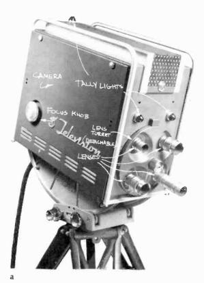
2.7 Vidicon Cameras: (a) RCA-TK 15 vidicon camera, a viewfinder studio camera; (b) General Electric industrial camera, a type used for closed-circuit observation; (c) Sony "portapak" camera, a highly portable camera used in conjunction with a small ½-inch videotape recorder.
