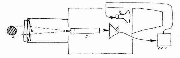
2.5 Basic Principle of Television Camera: (a) light reflected off object; (b) lens gathers light and focuses image of object onto front surface of pickup tube; (c) camera pickup tube with photosensitive surface that converts light into electrical energy, the video signal; (d) preamplifier, which strengthens signal; (e) electronic viewfinder, a small television set that shows what the camera is photographing. In most color cameras, the viewfinder produces only a blackand-white picture.
