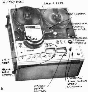
from the tape]), and *stop* (stops the reels almost instantly, depending on the quality of the reel brakes). Most machines have an additional *standby*, or *ready*, button, which makes the video heads rotate (getting them up to speed) before moving the tape. (See 9.13.)
