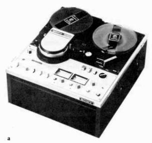
17·14 (a) Sony AV-8650  $\frac{1}{2}$ -inch Color Videotape Recorder has insert and assemble editing modes, as well as slow-frame and still-frame capabilities.
