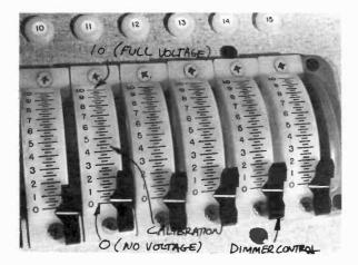
5.44 Dimmer Calibration: At a dimmer setting of 0, no current flows to the lamp; at a setting of 10, the full current flows to the lamp, and the lamp burns at full intensity.
