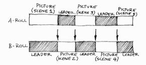
10.26 A-B Rolling: In A-B rolling, roll A is composed of all odd-numbered shots, separated by leaders that correspond exactly to the even-numbered shots; roll B is composed of all even-numbered shots, separated by leaders that correspond exactly to the odd-numbered shots.
