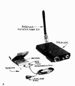
7.16 Wireless Microphones: (a) The wireless microphone has as its sound-pickup device a small lavaliere mike which is attached to a transmitter. A special receiving station receives the signal and sends it
