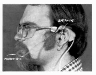
to be in voice contact wear telephone headsets with a small earphone and a microphone for talkback.
