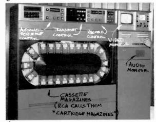
second roll) is now done by the cassette machine automatically, with ease and reliability. The cassette recorder selects the tape cassette, threads the tape, and cues it, within seconds. (The start button starts the tape roll and puts the picture "on the air" in one operation. No preroll is necessary for the cassette. The cassette recorder can record off any VTR, or another of its cassettes.
