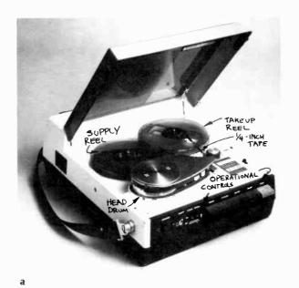
9·12 Helical Scan Videotape Recorders: (a) AKAI VT-150 (¼-inch portable color VTR; shoulder bag); (b) Sony AV-8650 (½-inch color recorder); (c) IVC-960 (broadcast-quality 1-inch helical scan color recorder); (d) IVC-9000 (top quality 2-inch helical scan high-band color recorder).
