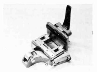
Film Tape Splicer: Contrary to the cement splicer, which welds the base sides of two pieces of film together with film cement, the tape splicer uses a piece of transparent tape for joining two pieces of film. The advantage of the tape splicer over the cement splicer is operational speed. No scraping is necessary, and there is no drying time for the cement. The film is cut and taped in one quick operation.
