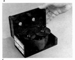
9.17 Videotape Cassette Machines: (a) Ampex ACR-25; (b) automatic sequence control for ACR-25; (c) 2-inch videotape cassette and tape; (d) RCA TCR 100-A. The 2-inch videotape cassette allows the back-to-back use of short videotaped program material, such as a series of consecutive 10-second spots. What would have been an impossible feat with two regular VTR's (loading, threading the tape, and starting the tape within five seconds, assuming a 5-
