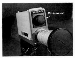
17-11 Most portapak cameras have an omnidirectional microphone attached or built in, pointing into the direction of the lens.
