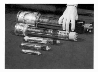
2.6 Television Pickup Tubes (from top to bottom): 4½-inch image orthicon; 3-inch image orthicon; 25mm Plumbicon; 1-inch vidicon; 2⁄3-inch vidicon.
