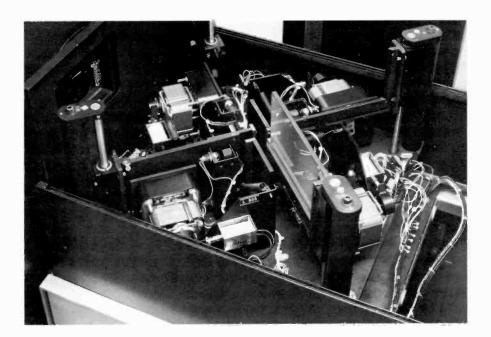
9.31 Multiplexer: The multiplexer consists of a series of mirrors or prisms that direct the light of the various program sources, such as film projectors or slide projectors, into the television film (also called telecine) camera.
