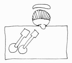
7.19 Dual-Redundancy Microphones: Two identical microphones can be used side by side, as long as only one is turned on; otherwise, multiple microphone interference will cancel out certain frequencies. The dual-redundancy system is used as a backup system, in case one of the two microphones fails during the telecast.
