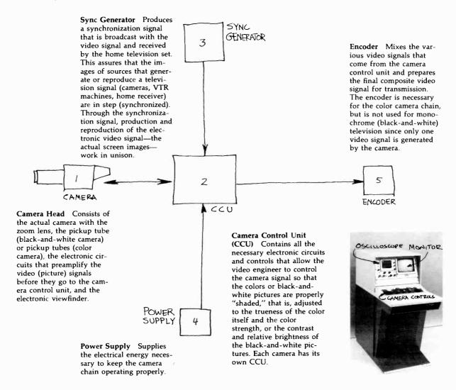
2.4 Camera Chain: The camera chain consists of (1) the camera head, which is what we ordinarily call the television camera; (2) the camera control unit, or the CCU; (3) the sync generator; and (4) the power supply. The color camera has an additional part, (5) the encoder.
