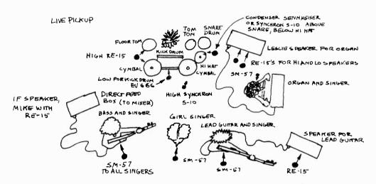
7.23 Microphone Setup for a Small Rock Group: When miking a rock group, you need microphones for the singers, drums, and other direct sound-emitting instruments, such as flutes and pianos, as well as for the speakers that carry the sound of the amplified instruments, such as electric guitars and organs. The microphones must be placed so that they do not cause audio feedback or multiple audio interference.
