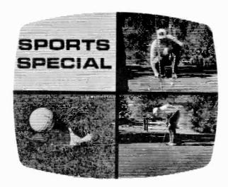
11-17 Some switchers permit a quad, or four-way, split. You can then fill each of the four screen areas with a different picture.
