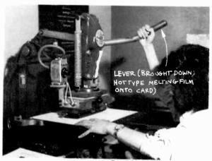
12·32 (a) First, lock the type in mirror image into the chase and preheat the whole thing on a special hotplate to approximately 250°. (b) Then insert the chase into the hotpress, whose head has also been preheated to the same temperature. (c) Line up the card underneath the chase and place the plastic film
