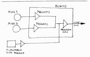
7.40 The weak sound signals that originate from a microphone or a turntable cartridge need to be boosted by a preamplifier, or preamp, before they can be controlled (as to volume, which is just like the loudness control on your hi-fi set) and distributed throughout the audio console. The preamplified signals are then amplified again by the program amplifier to make them strong enough for the line-out.
