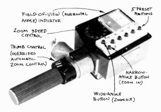
3.27 Shot Box: The shot box comes in a variety of configurations, but with similar components, such as the field-of-view meter, zoom speed control, wide-
