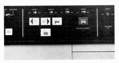
9-13 Operational Controls (Ampex AVR-2).
