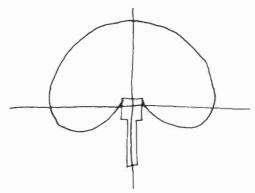
7.3 Cardioid Pickup Pattern: The most common unidirectional pickup pattern is called *cardioid*, heart-shaped. If you think of an apple with the mike sticking into it where the stem should be, you will have an idea of the three-dimensional pickup pattern of most unidirectional television microphones.<sup>1</sup>
