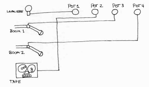
7.37 Patching: Lavaliere microphone patched into pot 1; boom microphone no. 1 into pot 3; boom microphone no. 2 into pot 4; and the tape recorder into pot 2.
