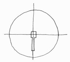
7.2 Omnidirectional Pickup Pattern: You can think of the omnidirectional pickup pattern as a large rubber ball with the mike in its center. All sounds that originate within the confines of the rubber ball (the pickup pattern) will be picked up by the microphone without any marked quality difference.
