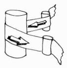
9.5 Helical, or Slant-Track, Scanning: In the helical, or slant-track, scanning process, the tape moves past the rotating heads (head drum) at an angle. Because the scanning occurs diagonally, it covers a longer area of the tape than its width.
