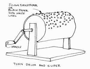
11.35 Rain: A rain drum consists of a small drum (about ten inches [25 cm] in diameter), covered with rough black sandpaper or black paper with white "glitches" painted on it. Turn the drum fairly fast (depending on how hard you want it to rain), take a slightly out-of-focus closeup of the rotating paper, and super the glitches over the scene. Make sure that you turn the drum so that the rain is coming down instead of going up.
