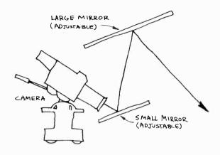
11-29 Periscope: The mirror periscope, consisting of two adjustable mirrors hung in a movable frame, permits a variety of overhead shots of fairly static scenes. When using it, you don't need to reverse the horizontal sweep in your camera, since the image will be corrected by the second mirror.
