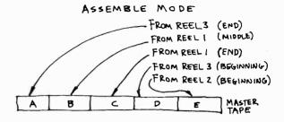
10-30 Assemble Mode Editing: In the assemble mode, any number of scenes can be assembled consecutively onto the master tape. But no inserts can be made without affecting the material that follows the desired insert.
