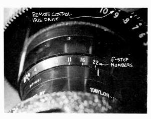
**3.6** /-Stop: The /-stop is a calibration that indicates how large or small the iris, or lens opening, is.
