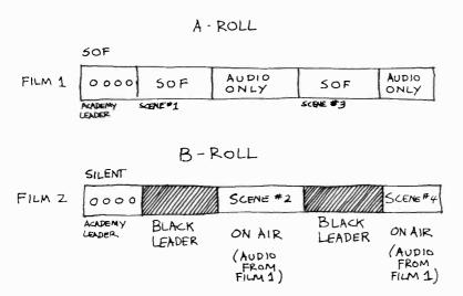
10.27 Electronic A-B Rolling: In electronic A-B rolling, the complete SOF interview is played on one film island (constituting the A roll). The silent shots, which are carefully matched to the narration and separated from each other by black leader whenever necessary (when the A-roll is on the air with video and audio), are played simultaneously on the other film island (constituting the B roll). You can switch to the B-roll video while resuming the A-roll audio.
