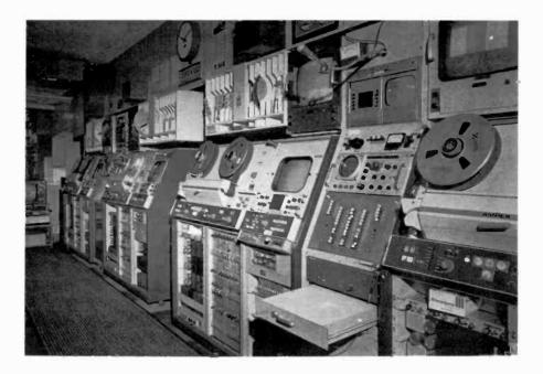
multaneously. Also, with all CCU's in one location, the test equipment does not have to be moved from one studio control room to another. (See 8.14.)
