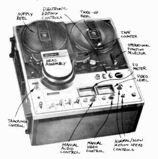
9.14 Controls for most helical scan VTR's include features, such as forward, fast forward, record, and stop. Some of the more advanced models have separate controls for slow motion and stop-motion, and stand-by (which starts rotating the video heads without moving the tape). The arrangement of the controls differs from model to model, but they fulfill identical functions. (Sony AV-8650.)
