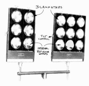
5-22 Floodlight Bank: The floodlight bank consists of at least six individual internal reflector lamps, stacked as two three-lamp strips. Larger banks stack three, four, or even five three-lamp strips for a total of nine, twelve, or fifteen internal reflector bulbs.
