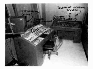
8-10 Lighting Control: The lighting control board consists of the dimmers and their preset controls, through which a variety of lights can be adjusted for their intensity either individually or in unison, depending on how they are patched.
