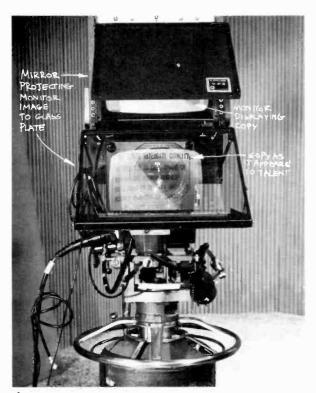
plate directly over the lens. (c) You can then read the copy without losing eye contact with the lens (the viewer). The advantage of this system is that a single copy can be displayed on two or more cameras.
