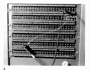
7.38 (a) Patch Panel: All major audio inputs terminate in the patch panel, or patchbay. Each piece of equipment that can be patched has an "in" and an
