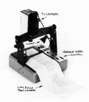
13.3 Television Prompting Device: (a) The copy, typed on a news typewriter with oversized letters, is placed in a special variable-speed crawl. A simple vidicon camera picks up the copy and relays it to a
