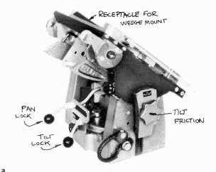
4.9 (a) Vinten Cam Head. (b) ITE Cam Head.
