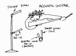
7.21 Microphone Setup for Singer and Acoustic Guitar: The customary way to mike a singer who is accompanying himself or herself on an acoustic guitar is to have two microphones on a single mikestand, such as an Electro-Voice RE-15 pointing at the guitar and a Shure SM61 pointing at just below the singer's mouth.
