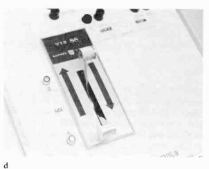
10.5 (a) With both fader bars in the up position, B bus is activated. (b) With both fader bars in the down position, A bus is activated. (c) With the fader bars split, with fader bar B in the B bus position and fader bar A in the A bus position, both buses are activated. If a video source is punched up on either bus, we will have a superimposition. (d) With the fader bars split against their direction (the B bar
