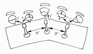
7.20 Multiple Desk Microphone Setup: When using a multiple-microphone setup, you should keep the individual microphones at least three times as far apart as any microphone is away from its user.
