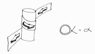
9.6 Alpha Wrap: If the tape has to be wound completely around the head drum, we speak of an alpha wrap, because the wind suggests the configuration of the Greek letter  $\alpha$ .
