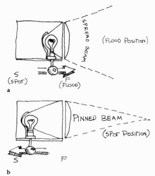
5.8 Beam Control of Fresnel Spotlight: (a) In order to spread the beam, turn the focus spindle or focusing loop so that the bulb-reflector unit moves toward the lens. If the lighting instrument has an outside indicator, the indicator should move toward F (for "flood" position). (b) In order to pin, or focus, the beam, turn the focus spindle or focusing loop so that the bulb-reflector unit moves away from the lens. The focus indicator should move toward S (for "spot" position).
