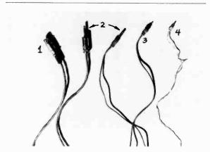
17.12 There are generally four major types of audio cable connectors: (1) the Cannon connectors, (2) the phone plug, (3) the RCA plug, or phono plug, and (4) the mini plug.
