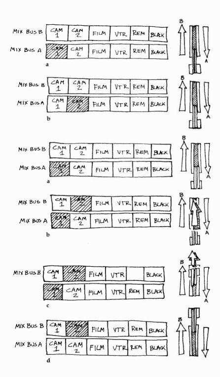
10.11 (a) With the A bus activated (both fader bars are down), the camera 1 button will put camera 1 on the air. (b) By pressing the camera 2 button, you accomplish a cut from camera 1 to camera 2.
