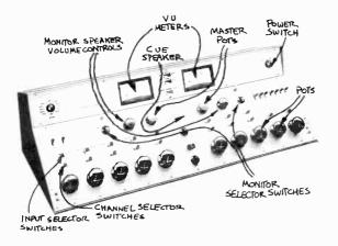
7-47 Audio Console: (a) A traditional audio console (RCA BC-7 Audio Consolette). (b) A four-channel
