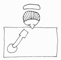
7.18 Desk Microphone for Single Performer: When using a desk mike, put it to the side of the performer (if he uses a floor monitor, put it to the monitor side, since a person will be more apt to speak toward the monitor than the opposite side) so as to maximize the camera view, and pointed up toward his collarbone so that he will speak across the mike rather than directly into it. If the talent uses his desk a great deal, put the microphone on a soft pad to absorb at least some of the shocks.
