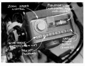
angle and narrow-angle zoom buttons, and buttons for preset positions.
