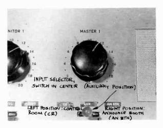
7-39 Input Selector Switch: Most input selector switches are of the three-position type, which means that you can choose among three different audio inputs. In this case, you have a choice among control room (CR), auxiliary (AUX), and announce booth microphone (AN BTH).
