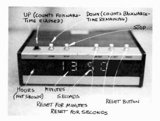
8-6 Digital Stopwatch: The digital stopwatch is an extremely helpful production tool. In the up, or forward position, it indicates the elapsed running time in hours, minutes, and seconds. You can set the watch for any given time, stop and start it at any given point, and reset it to zero. In the down, or reverse position, the watch shows time remaining. If you have three minutes left in your show, the stopwatch will show 3:00 on the dial. When it shows 0:-00:00, you should be off the air.
