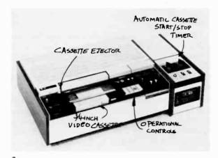
9.18 (a) Sony U-matic VO-1800 ¾-Inch Video Cassette and Timer: The ¾-inch helical scan cassette machine can hold cassettes with up to one hour of program material. It has automatic cuing and preroll, and can record material from a direct source, such as
