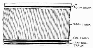
9.2 The 2-inch videotape for quadruplex videotape recorders normally has four tracks: the video track (television pictures), the audio track (television sound), the cue track (various code information or a second audio track), and the control track (essential for synchronization).
