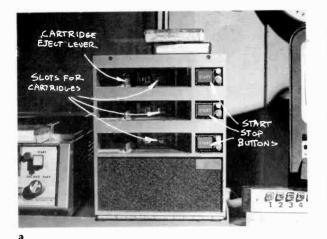
7.35 (a) Three-Unit Cartridge Machine. (b) Cartridge.
