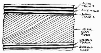
9.4 Two-Inch Helical Scan Videotape: The highly sophisticated 2-inch helical scan videotape has a total of six tracks: the slanted video track, two audio tracks, a cue track, an additional address code track, and a control track.
