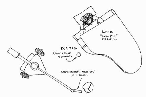
7.22 Microphone Setup for Singer and Piano: A singer who is accompanied by a piano might be miked with a Sennheiser MKH-415 (or even an 815) suspended from a boom. There could be an RCA 77-DX for the piano, placed just above the strings on the highstring side, with the lid in the low-peg position (half open). The formality of the recital probably forbids the use of a hand microphone.
