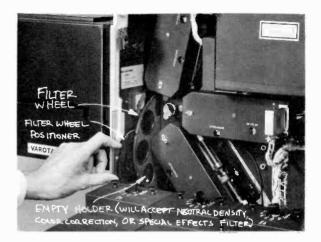
2.12 Filter Wheel: The filter wheel can hold a variety of neutral density or color correction filters. In some cameras, the filter wheel can be turned by remote control.
