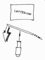
12:34 If the lettering is high on the left, rotate the easel counterclockwise.
