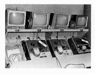
(b) Editing Bench, using Sony AV-3650 ½-inch Monochrome Videotape Recorders.
