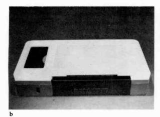
cameras, the television set, or from any standard playback device of recorded material (film chain, VTR). The ¾-inch cassette is the slant-track cassette standard. (b) A typical ¾-inch cassette.
