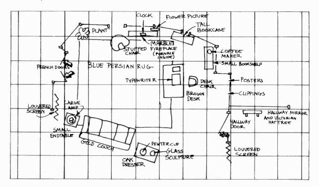
12.44 The completed floor plan shows the exact location of the scenery and set properties, relative to the lighting grid or pattern of battens. The floor personnel use this plan as a guide for setting up the scenery and placing the major properties.
