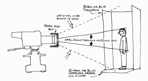
11-33 Matte Box: With the aid of a matte box, you can isolate an object in an extreme long shot without overshooting the set. This technique is especially important if you want to reduce the size of an object or performer for chroma key matting.
