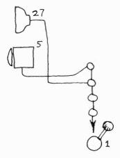
5.45 Patching: As you can see, the patches for the lighting instruments No. 5 (spot) and No. 27 (scoop) are both patched into dimmer No. 1. Consequently, both lighting instruments respond identically to any No. 1 dimmer setting.
