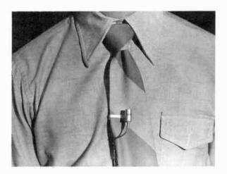
7.13 Correct Lavaliere-Microphone Position: This lavaliere mike is properly attached for maximum sound pickup. It is securely fastened *on top* of the clothing, minimizing the danger of causing highly distracting rubbing noises. The mike cord is concealed. In spite of its small size and its distance from the sound source, the quality of sound pickup in this small microphone is excellent.
