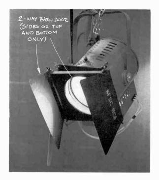
5.42 Two-Way Barn Door: The two-way barn door has two movable metal flaps. They can be attached to the lighting instrument so that they block either the top and bottom part of the light beam or its right and left spread.
