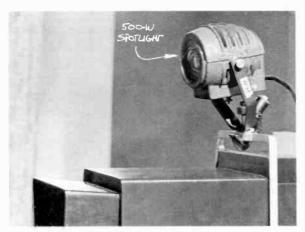
6.9 Camera Light: A small spotlight is sometimes mounted on the camera to provide additional fill light, highlights (to add sparkle to eyes, for example), or general illumination for easel cards.
