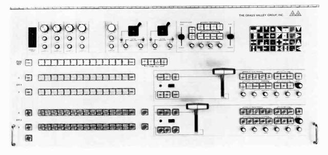
10.8 Large Grass Valley Production Switcher: On large production switchers, the various switching modes can be assigned to the buses, such as preview and key (top bus) and effects and mix (effects 1 and 2 buses).
