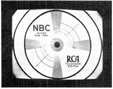
FIG. 68b.—The standard test pattern as reproduced by television.
