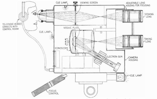
FIG. 24,-Cross-sectional diagram of a television camera used in studio productions.
