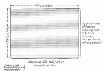
FIG. 61.—Some television standards associated with the physical dimensions of the picture.
