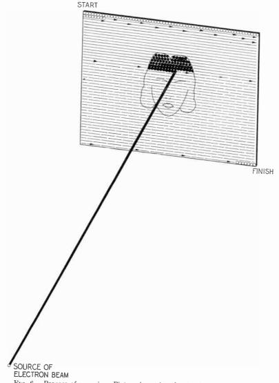
FIG. 6.—Process of scanning: Picture is analyzed point by point in a definite sequence, the amount of light associated with each point registering a corresponding influence on the transmitted radio signal. At the receiver, the process is virtually reversed.
