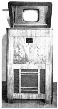
F16. 9a.—A model of receiver used during the field-test period of the development of the RCA-NBC television system.
