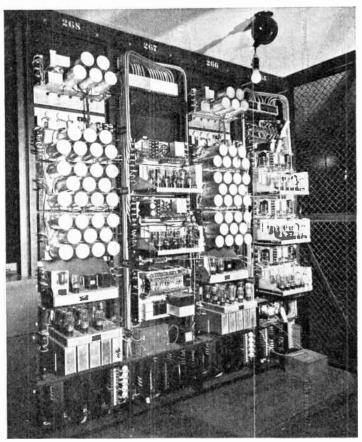
FIG. 17.—Part of the apparatus "behind the seenes." These are the synchronizing signal generators which form the heart of the television system. They create the timing impulses which keep the receivers and transmitter working in unison.
