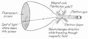
FIG. 8.-The principal parts of a Kinescope,
