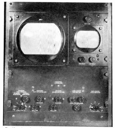
FIG. 19a.—A monitor used in the control room. The larger of the two screens is equivalent to a home-type receiver, and the smaller is the screen of an oscilloseope which shows the engineers the electrical equivalent in the form of a wave shape of the actual image being observed. By observing both of these screens the engineers adjust the television signal to insure best reception in the home.
