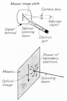
FIG. 63.—The essentials of the Iconoscope. Also, the existence of secondary electrons is shown diagrammatically.
