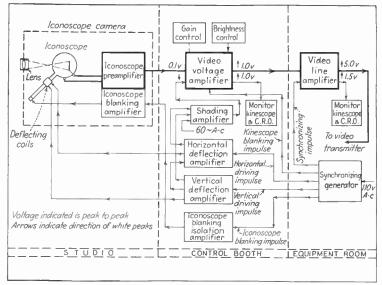
FIG. 67.—A typical one-channel television system.
