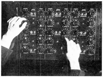
FIG. 64,—The shading panel in the control room,
