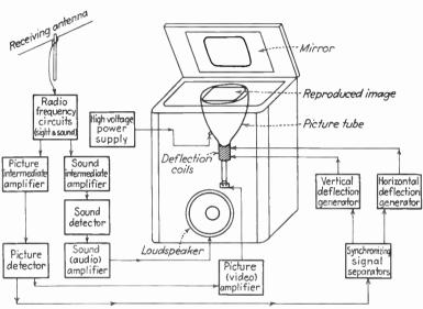
FIG. 72 .--- Diagram of the principal parts of a television receiver.
