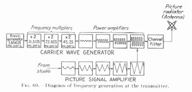
munications Commission. A similar arrangement is used to obtain a carrier wave of 49.75 Mc. per second, which is used to carry the sound signal associated with the picture.
