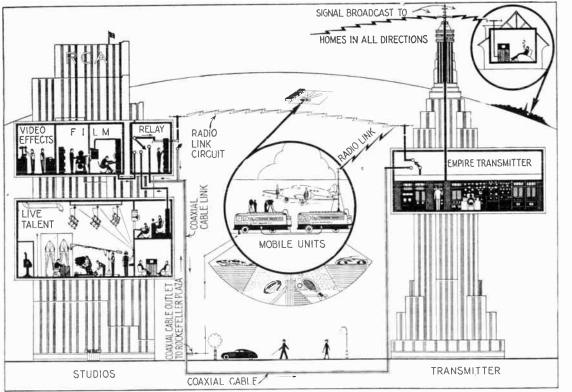
FIG. 20.—The three sources of program origination; live talent, film, and outside pickups; and the methods used to relay the television signal to the main transmitter at the Empire State tower for rebroadcast to viewers in the  $\Im$  New York area.
