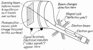
FIG. 5.-The essential parts of an Iconoscope.
