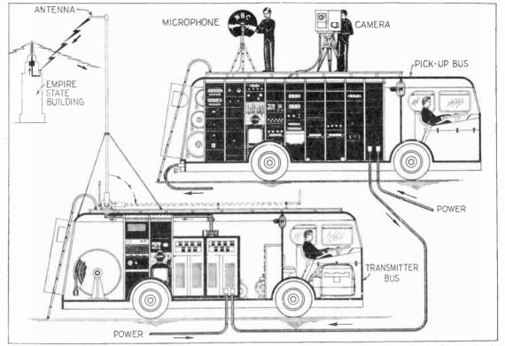
Fig. 44.- The television mobile unit. The upper unit is equivalent to a studio control room; the lower unit contains the radio transmitter used to relay the television signal to the Empire State Building for rebroadcast on the main transmitter.
