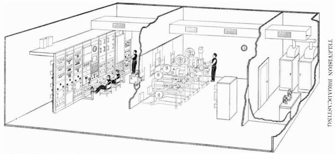
Fig. 33.—The projection studio at Radio City. From left to right, control room, projector room, and film vault and editing room.
