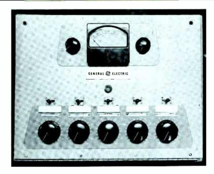
The General Electric BC-15-A audio console, showing VU meter. (Courtesy General Electric)
