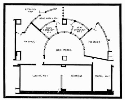
Unusual D-shaped studio layout at WDRC, Hartford, Connecticut. The main control for the combined AM/FM facility is at the hub of operations.
