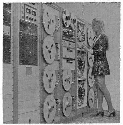
A traffic girl loading a cartridge into a carousel in the Schafer Model 8000 broadcast automation system.
