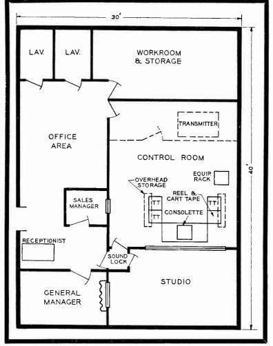
Basic floor plan designed by RCA for a minimum investment facility.
