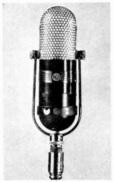
RCA all-purpose microphone Type 77-C. By turning the switch to line up the pickup pattern desired, it may be used for bi-directional, uni-directional, or non-directional purposes. (Courtesy of RCA.)
