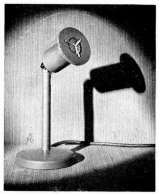
With the disk-shaped baffle applied, the 633-A microphone becomes a directional unit, and by means of the convenient universal joint it may be literally aimed at the sound source it is desired to pick up, effectively shutting out sounds from other directions. Without the disk-baffle, this microphone becomes a non-directional unit by returning it to a vertical position. (Courtesy of Western Electric Company.)
