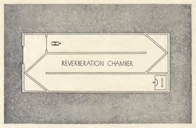
Figure 34. Labyrinth reverberation chamber.
