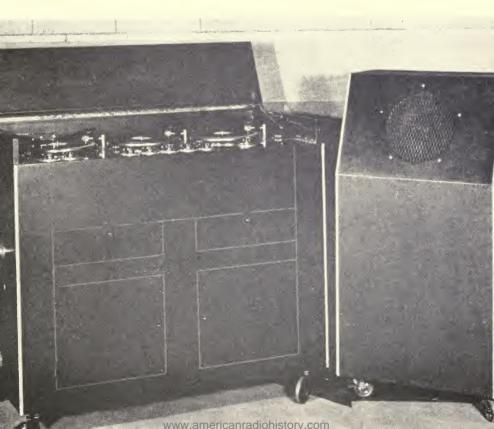
noise. The pick-up arms should be mounted so that they may be used on adjacent turntables. This will make possible the cross-fading from one pick-up to another to be used on the same record, in order that short cuts on a record may be utilized for longer sequences.
