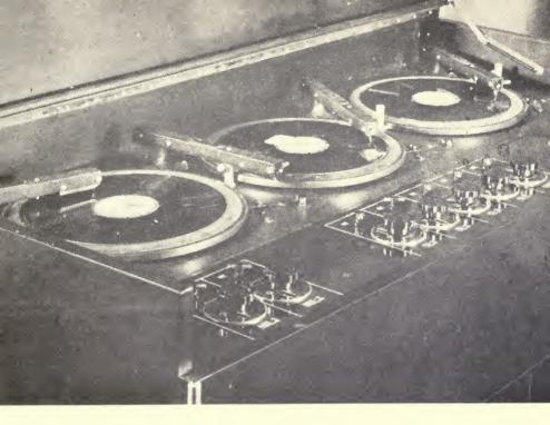
Figure 46. Turntable-speaker combination (bottom). Close-up of turntables (top).
