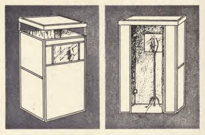
Figure 26. Booth constructed with acoustic screens.
