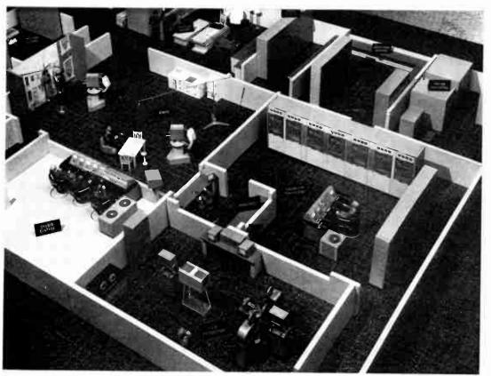
Figure 1. Typical Plan of One-Studio Television Station, with a two-camera studio and complete "two-film" camera projection room
