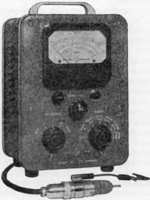
Fig. 1-2. Laboratory-type vacuum-tube voltmeter. This instrument is designed to measure a-c, d-c, and r-f voltages up to about 200 megacycles.
