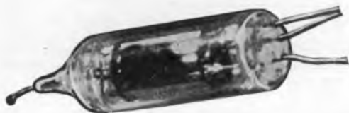
Fig. 9-4. The 1247 duo-diode sub-miniature, a common tube used in r-f probes.
