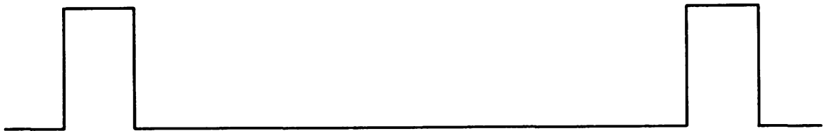
Figure 12. Waveshape of Current Through, Voltage Across, and Power Delivered to Resistor of Fig. 11
