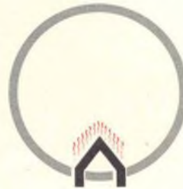
The heater heats the cathode
