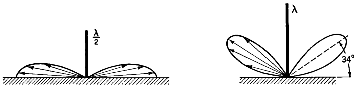
FIG. 8 E. Radiation patterns from vertical Marconi antennas
