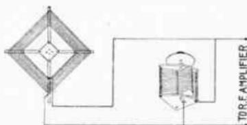
The Loop or Coil Antenna Tuner Unit.
