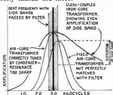
How Various Types of Intermediate-Frequency Transformers Function
