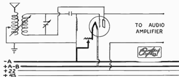
Here also we have a very sensitive hook-up, and one which is not expensive to build. Selectivity is naturally better than with the single-circuit, since but little energy is transmitted by inductive coupling except when the circuits are tuned to resonance. The interfering action, due to action of the tube as a generator, is not so bad as with the single-circuit, but requires very careful watching, and it is better to avoid the ultra-audion entirely in a crowded neighborhood.
