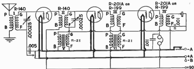
A very highly selective, long-distance Reflex receiver, with three stages of radio frequency amplification, followed by two audio frequency stages.
