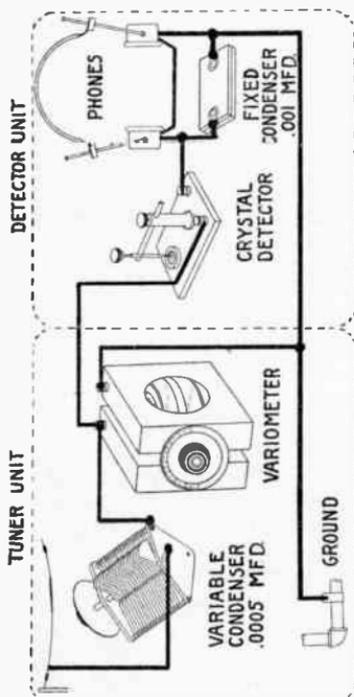
The crystal receiving set, as is well known, has only a short distance range, but it requires no batteries and gives a very good quality of tone. Ordinarily it will not operate a loud speaker, unless very close to a powerful broadcasting station, but its output can always be amplified if desired. This is done by simply removing the phones and the by-pass condenser, and connecting in the input leads of a good audio amplifier, such as shown on page 23.
