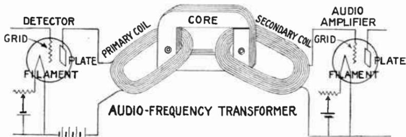
Transformer Construction: The Electric and Magnetic Links
