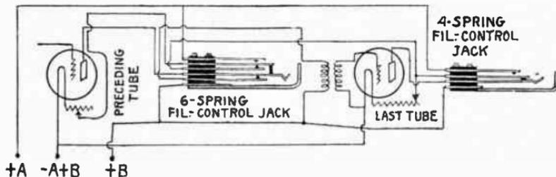
Wiring for Filament Control Jacks
