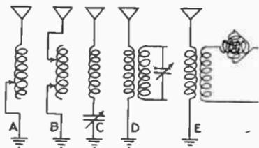
Different Methods by Which a Coil can
