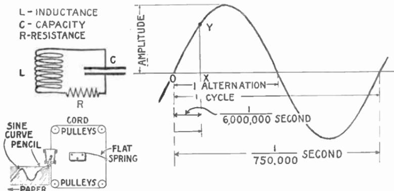
To the Left, An Oscillating Electric Circuit, with an Oscillating Mechanical Circuit Drawn Underneath for Comparison. To the Right, an Electric Current Wave.
