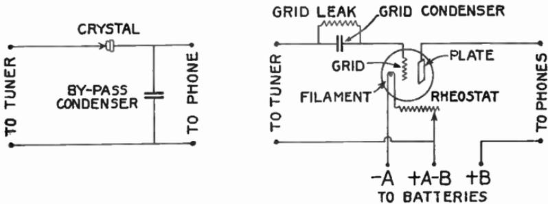
Detector Units: Crystal and Vacuum Tube Types
