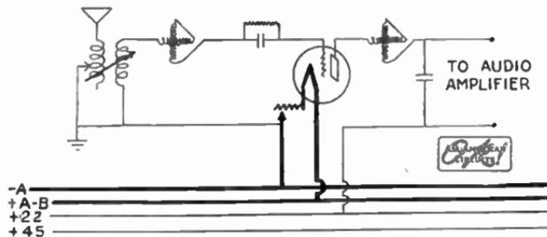
This is one of the "old original" regenerative circuits. The variometer in the plate circuit enables it to be tuned to the proper relation to the grid circuit so that regeneration will take place. The second variometer, in the grid circuit, tunes this circuit to the received signal. Selectivity is fairly good, as a rule. This circuit can be used with a loop antenna for local stations.
