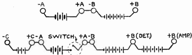
Battery Units: With and Without the Grid Battery
