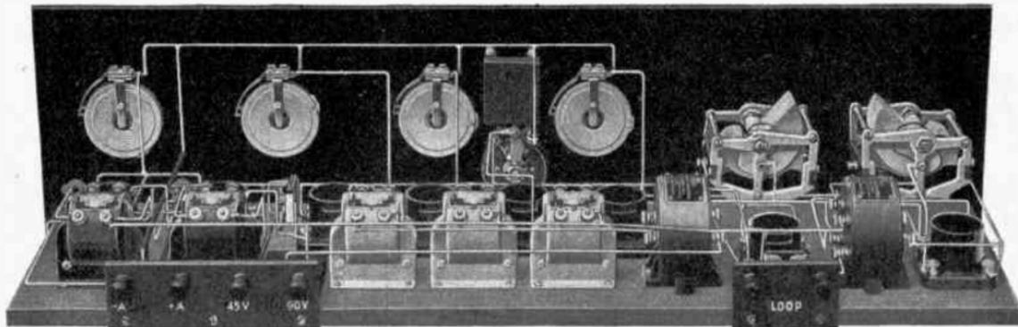
An Eight Tube Thirty Kilocycle Super-Heterodyne Receiver of Advanced Design, Utilizing the All-American Radio Frequency Coupler, 10,000 Meter Transformer, Long Wave Transformers, Standard Audio Transformers, and Tube Sockets. A Wiring Diagram of this Set Will be Found on Page 47
