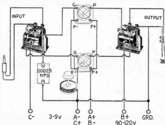
Complete Circuit Diagram for the Power Amplifying Stage
