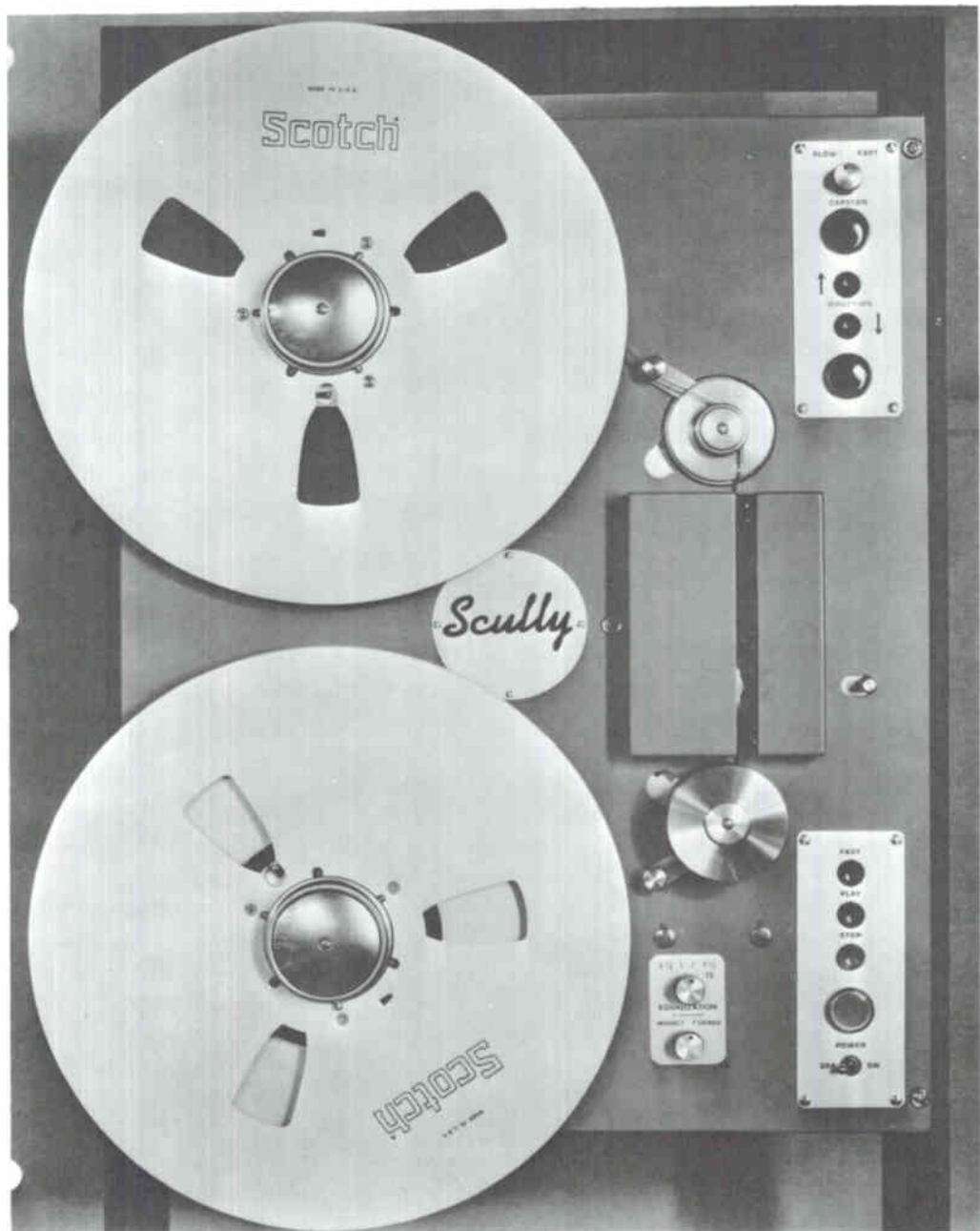
Fig. 11-7. Reel-to-reel mono or stereo tape playback unit.
