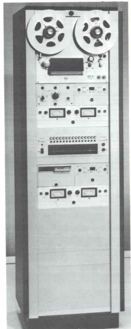
Fig. 11-9. This automatic audio system uses a stereo reel-to-reel recorder, (top) an automatic tape programmer, and a cartridge tape system.
