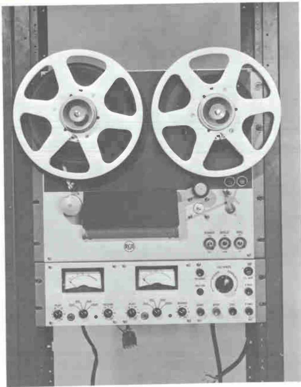
Fig. 11-4. A basic reel-to-reel audio tape recorder installed in a rack.
