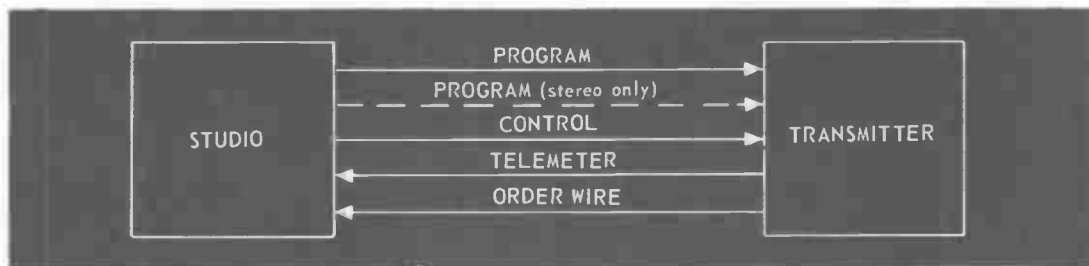
Fig. 9-6. Block diagram showing other STL remote control functions.
