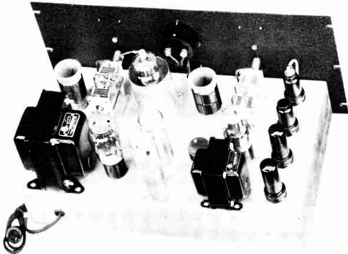
93. Rear view of Stancor 20-P Transmitter with cabinet removed
