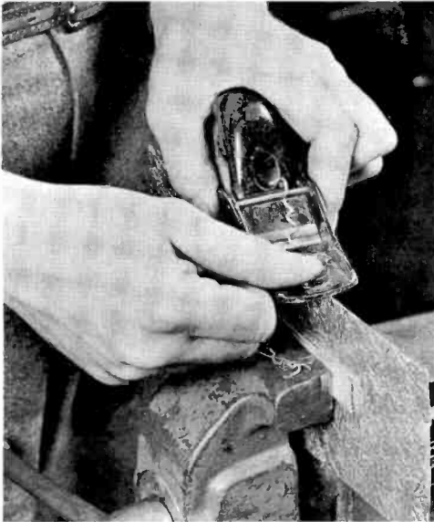
Figure 4 A WOODWORKING PLANE MAY BE USED TO SMOOTH OR TRIM THE EDGES OF ALUMINUM STOCK.
