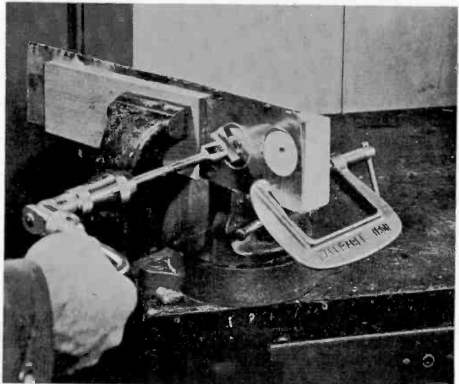
Figure 2 CONVENTIONAL WOOD EXPANSION BIT IS EFFECTIVE IN DRILLING SOCKET HOLES IN SOFT ALUMINUM
