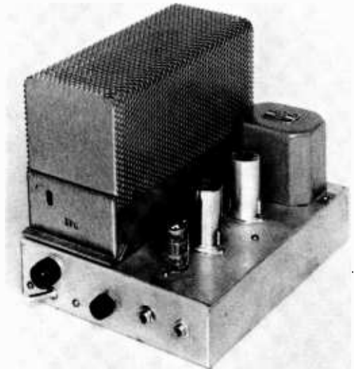
Figure 10 POWER SUPPLY-MODULATOR UNIT FOR THE 12-WATT TRANSMITTER
