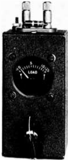
Figure 33 SIMPLE SILICON CRYSTAL NOISE GENERATOR
