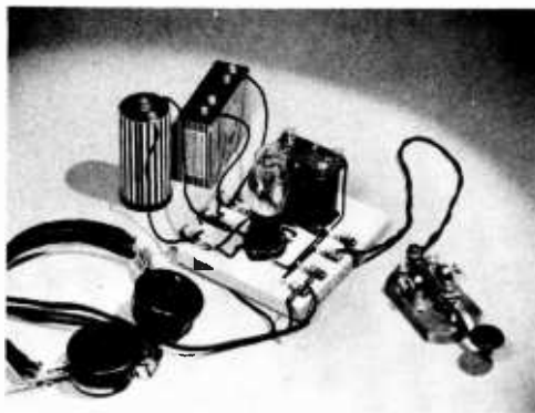
Figure 7 THE CIRCUIT OF FIGURE 6 IS USED IN THIS BATTERY-OPERATED CODE PRACTICE OSCILLATOR
