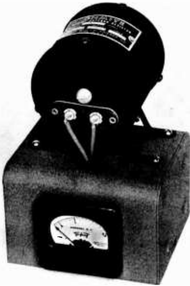
Figure 7 100-WATT DUMMY LOAD SUITABLE FOR VIKING II, OR SIMILAR TYPE TRANSMITTER
