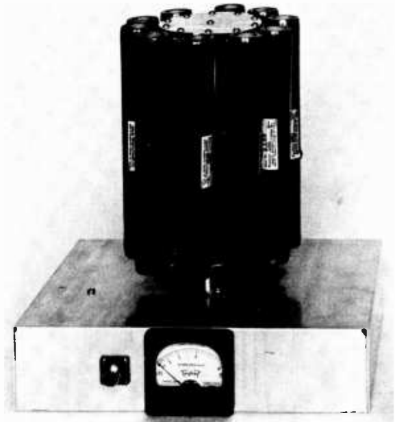
Figure 8 1600-WATT DUMMY LOAD, WITH EN- CLOSURE REMOVED
