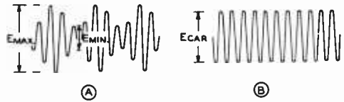
Figure 2 GRAPHICAL DETERMINATION OF MODULATION PERCENTAGE
