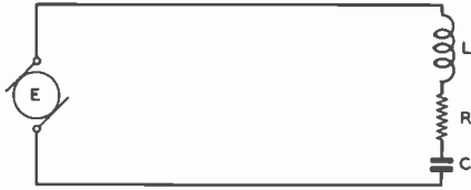
Figure 14. SERIES RESONANT CIRCUIT.
