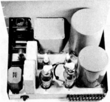
Figure 13. TOP OF THE TRANSMITTER MAIN POWER SUPPLY.
