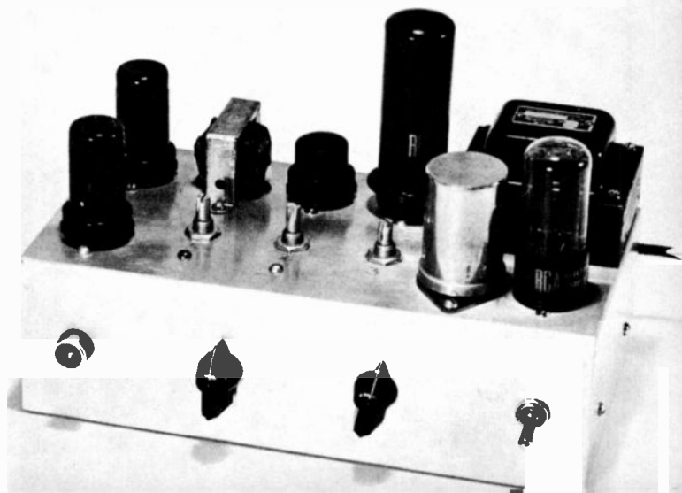
Figure 20. FRONT VIEW OF THE SCREEN MODULATOR UNIT.
