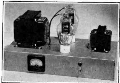
Figure 12. The class B 809 modulator with multiple-ratio input and output transformers.
