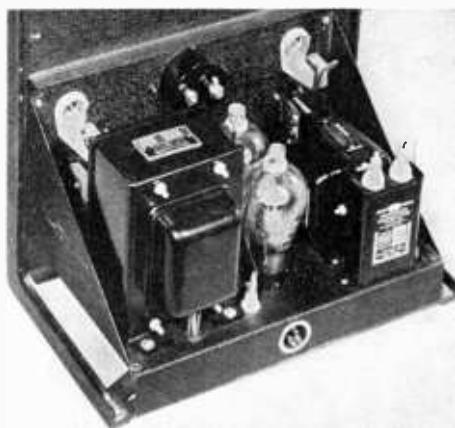
Figure 4. ILLUSTRATING ARRANGEMENT OF POWER SUPPLY COMPONENTS.
