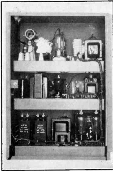
Figure 12. COMPLETED TRANSMITTER HOUSED IN CABINET, REAR VIEW WITH DOOR OPEN.
