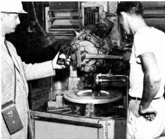
Figure 5-1. The Sound-Survey Meter being used for a preliminary investigation of machine noise.
