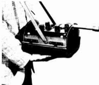
The sound-level meter is here operated while in its leather carrying case, with the microphones in the horizontal operating position.
