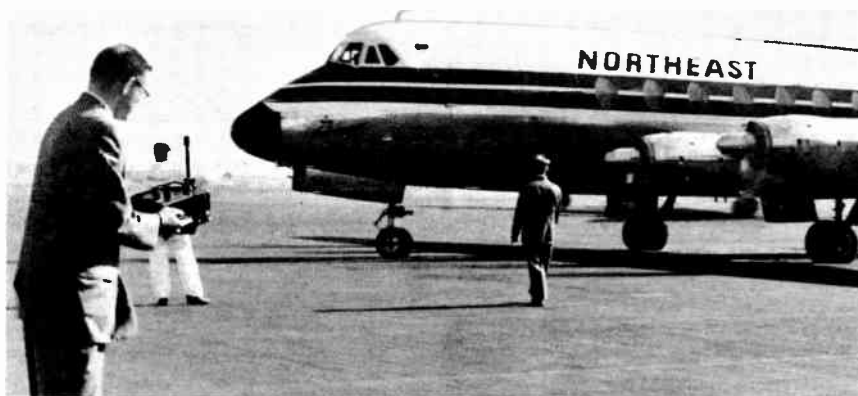
Figure 5-4. Sound-level meter being used to check noise at flight line.
