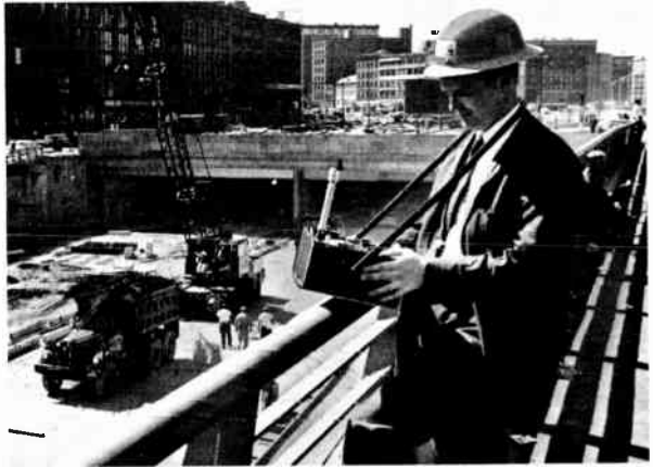
Figure 5-6. Another example of the sound-level meter in use: measuring noise level at a construction site.
