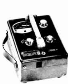
The Type 1551-C Sound-Level Meter with the microphone in the storage position and batteries automatically disconnected.
