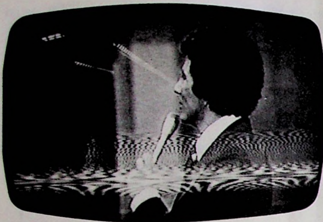
Fig. 13-22. Low frequency transistor radiation.
