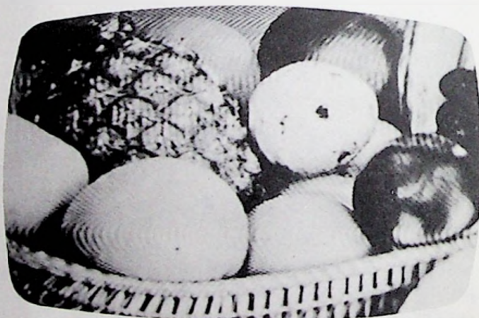
Fig. 13-19. Channel 8 tweet interference.
