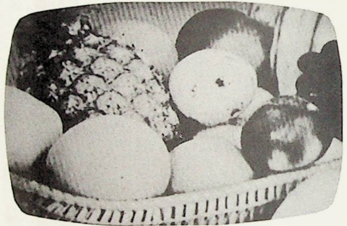
Fig. 13-4. Interference from am broadcast.
