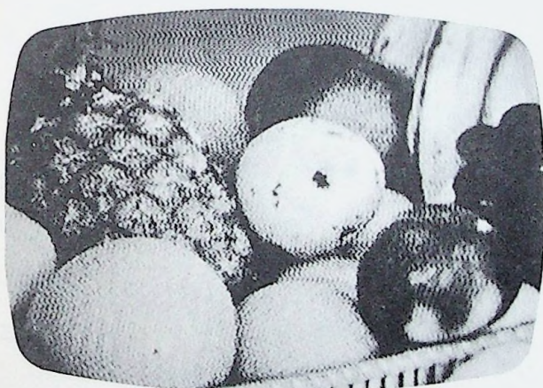
Fig. 13-10. Fm broadcast interference.
