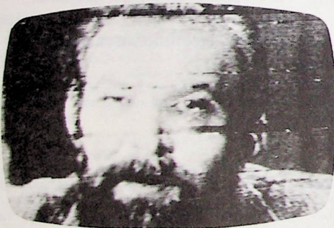
Fig. 13-13. Slip-ring noise interference.
