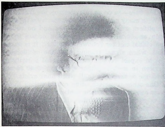
Fig. 9-30. When sound if signals beat with video signals a beat pattern such as this appears on the screen.
