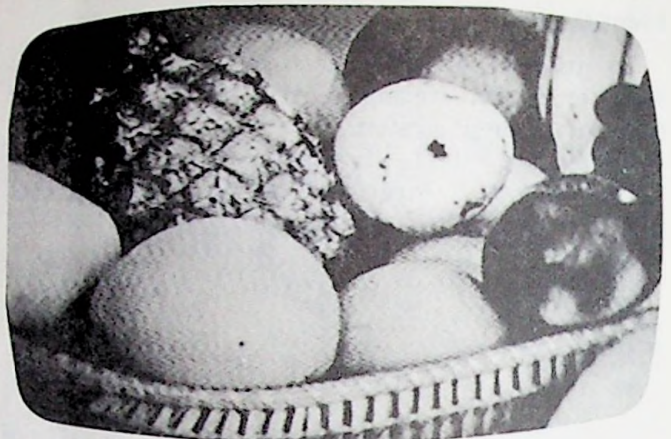
Fig. 13-8. Adjacent sound interference.
