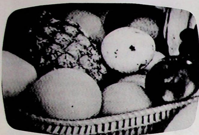
Fig. 12-37. Adjacent channel interference.
