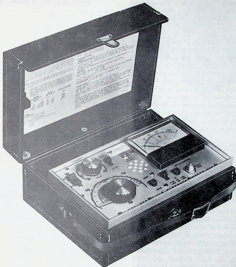
Fig. 12-17. Field-strength meter. (Courtesy Blonder-Tongue Laboratories, Inc.)
