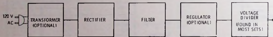
Fig. 3-17. A simple power supply (half wave).
