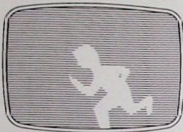
Fig. 4-3. A picture produced by scan lines.
