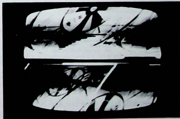
Fig. 6-31. Loss of vertical and horizontal sync.
