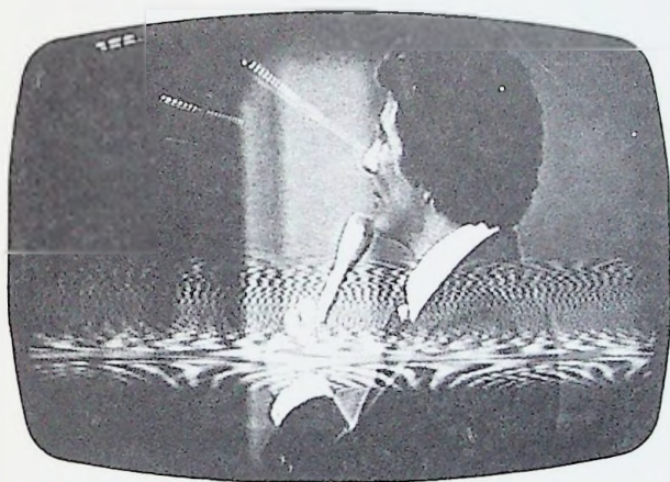
Fig. 13-15. Interference due to diathermy.
