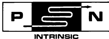
Fig. 8-4. Radio-frequency energy passing through a PIN diode.
