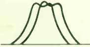
Fig. 2-5. Double RF response curve caused by improper setting of phasing control (no blanking used).
