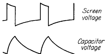
FIG. 168. Waveforms of screen voltage and voltage across the capacitor in the circuit of Fig. 167a.
