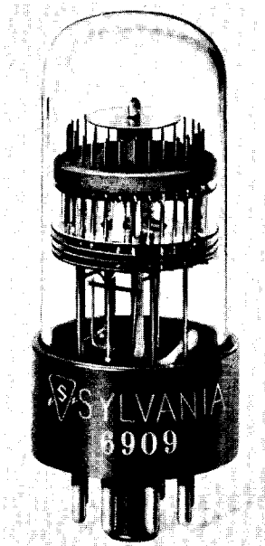
Fig. 136. Multiple-cathode counting glow tube. (Courtesy of General Telephone and Electronic Labs., Inc.)
