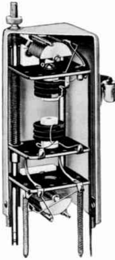
Fig. 12-34 Variable-coupling i-f transformer used to adjust the width of band-pass. (Hammarlund Manufacturing Company, Inc.)
