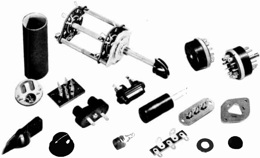
Fig. 4-1 Electronic applications of insulating materials. (P. R. Mallory & Co., Inc.)
