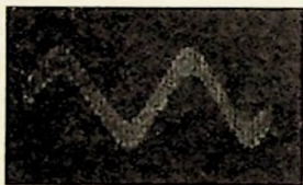
FIG. 40. WHEN THE HARMONIC FREQUENCY IS VERY HIGH THE WAVES DO NOT INTERACT
