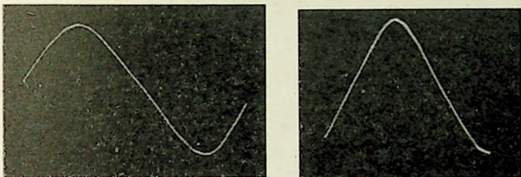
FIG. 51. EFFECT OF PHASE OF SYNCHRONIZING VOLTAGE ON SHAPE OF WAVE
