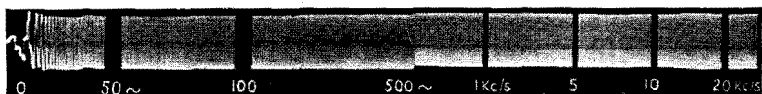
FIG. 17/4.—Response characteristic of final version of Garner Amplifier (without pre-amp). Note absence of peculiarities exposed in Fig. 17/3 which was taken under similar conditions, which proves that the Garner Amplifier is not as bad as it could be. The response is flat up to 35 Kc/s (see Fig. 17/11 for 20–40 Kc/s).
