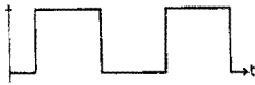
FIG. 1/4.—Square Wave. Note that the changes are extremely rapid, as shown by the vertical edges of the pulse.
