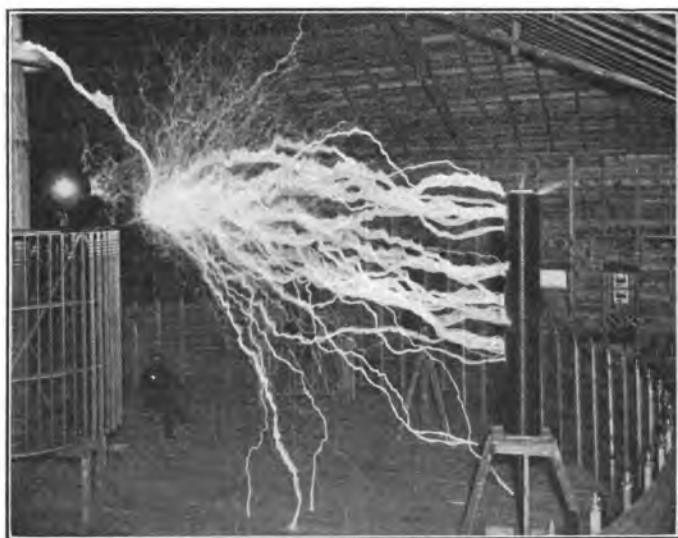
FIG. 156.—Twenty-five foot sparks from a Tesla transformer.
