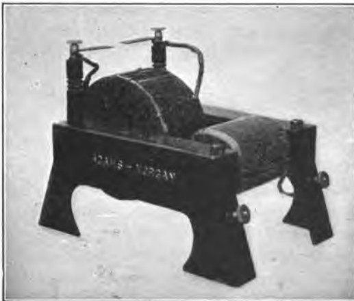
FIG. 43.—High potential closed core transformer for wireless work.
