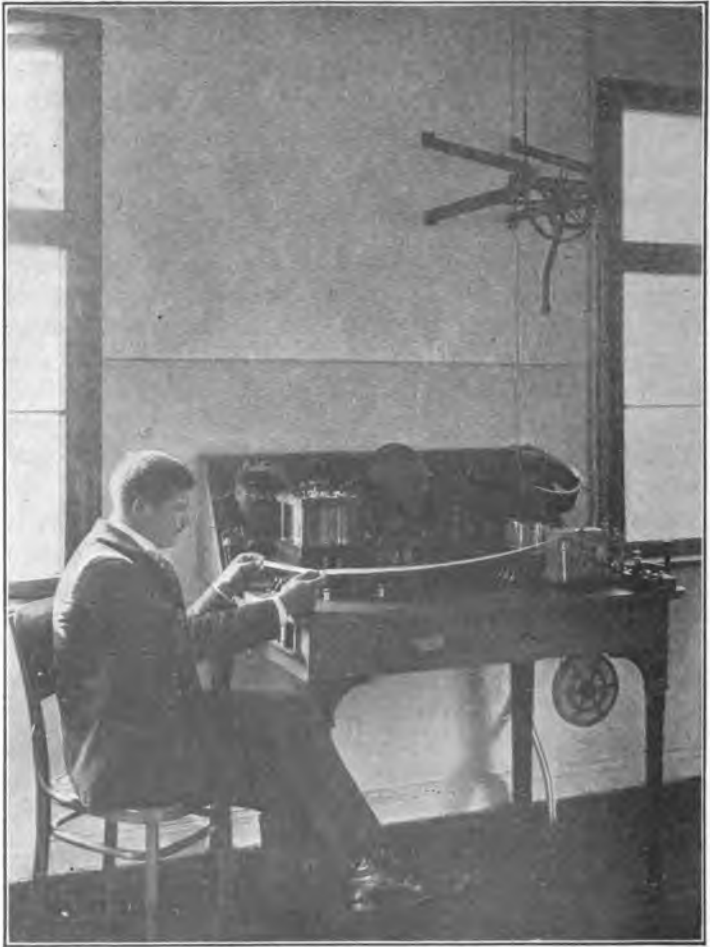
FIG. 119.—The receiving apparatus of the station at Nauen. The message is being printed on tape by a recording device.
