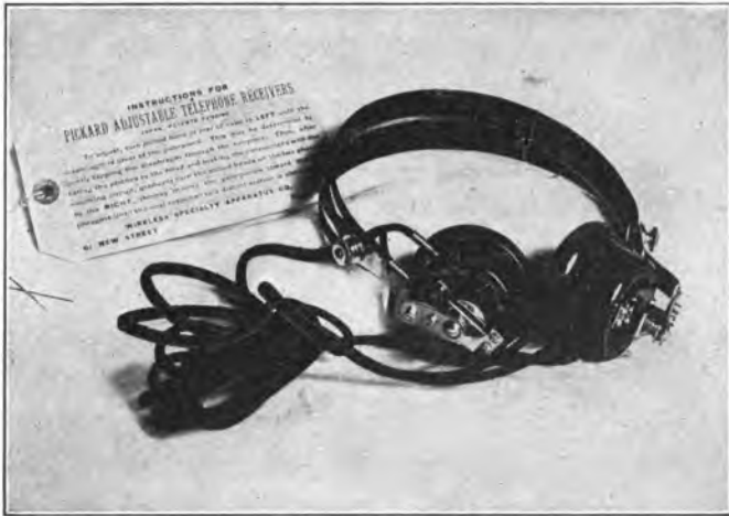
FIG. 65.—Pickard adjustable telephone receivers for wireless purposes.
