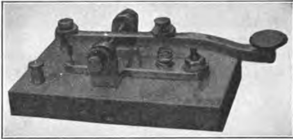
FIG. 58.—Photo of wireless key.
