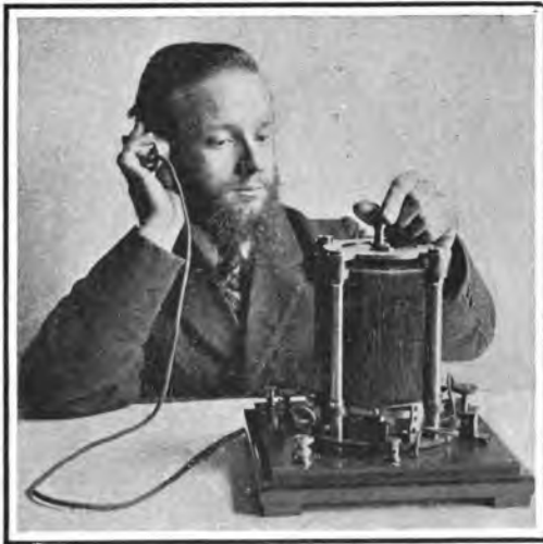
FIG. 97.—Bellini-Tosi radio-goniometer for directive wireless telegraphy.
