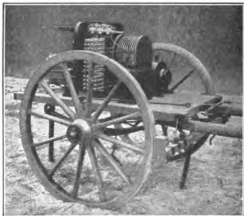
FIG. 101.—Telefunken wireless cart, showing transmitter.
