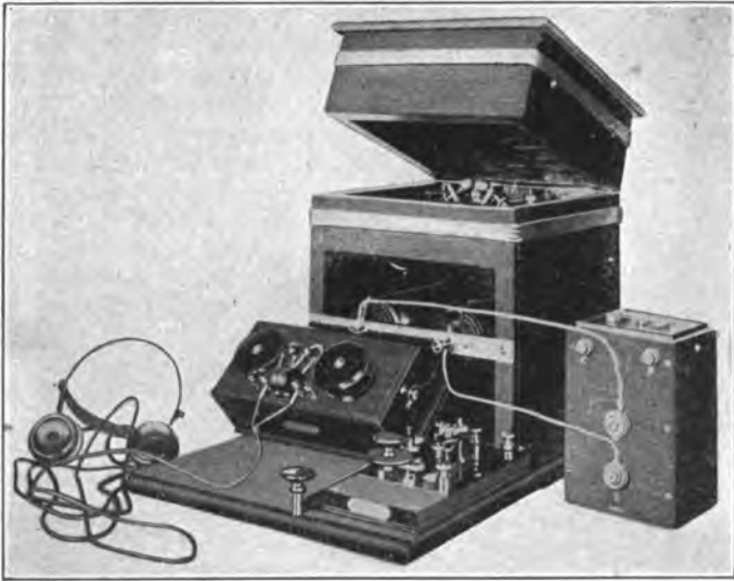
FIG. 109.—The receiving apparatus of the airship "America" (Wellman expedition).
