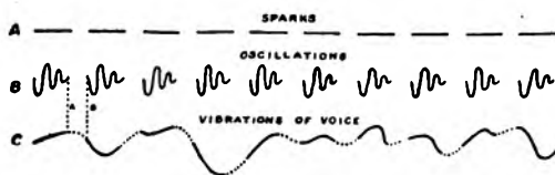
FIG. 143.—Diagram illustrating the reason why damped oscillations will not carry the voice.
