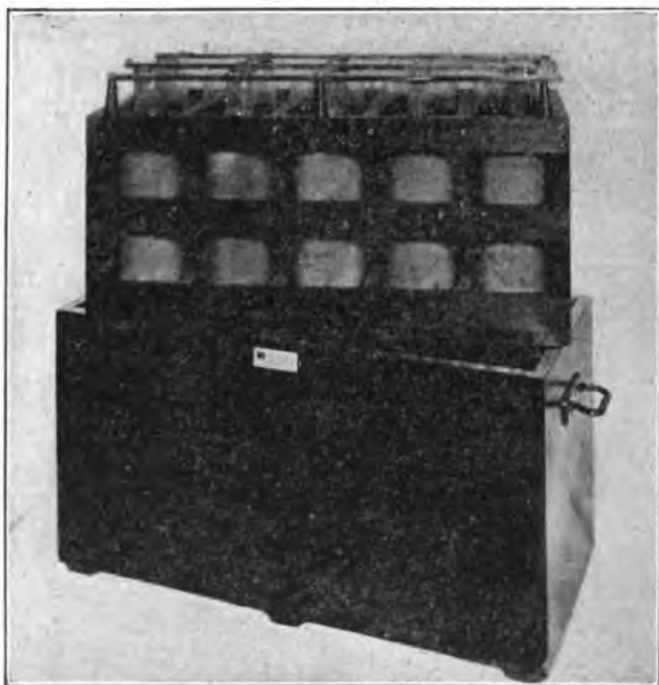
FIG. 44.—Leyden jar set for oil immersion to prevent losses from brush discharges.
