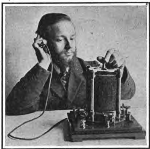
FIG. 97.—Bellini-Tosi radio-goniometer for directive wireless telegraphy.
