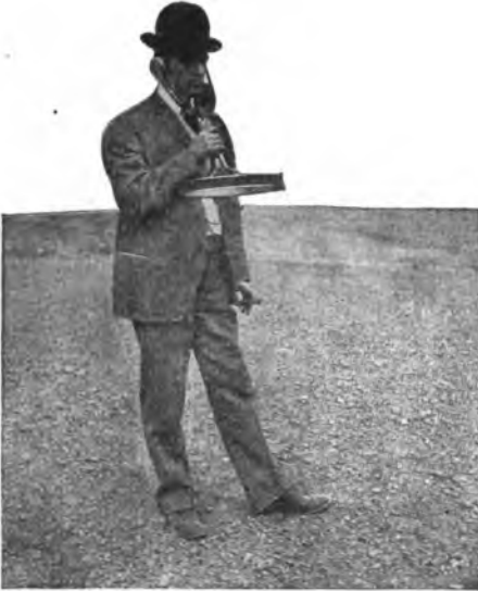
FIG. 141.—Wireless telephone receiving apparatus (induction method).
