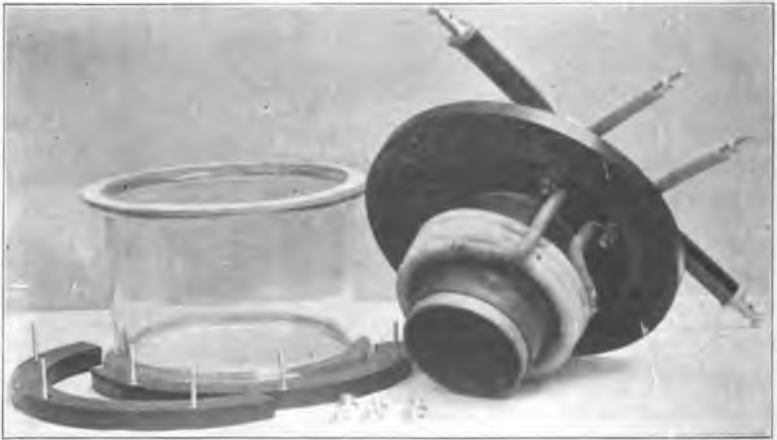
Braun High Potential Transformer.
