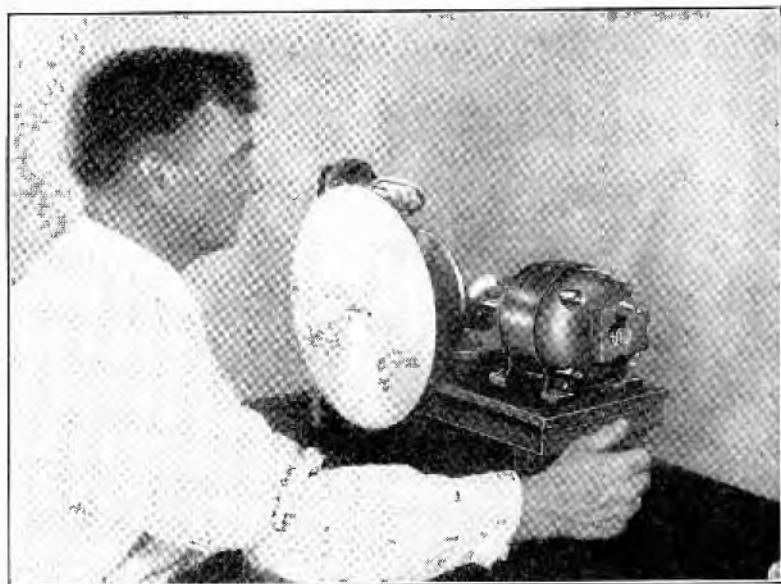
FIG. 324. Experimental Scanning Disc Arrangement and Driving Mechanism.
