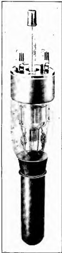
FIG. 108. Western Electric 5-K W. Water-Cooled Power Tube.
