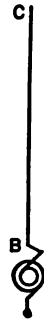
FIG. 2.—Without the lower wire the capacity of the condenser is so small that the alternator could not force an appreciable current to flow in the upper wire.
