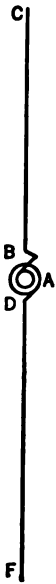
FIG. 1.—Theoretically the simplest type of antenna, the two wires CB and DF form the two plates of an open condenser.
